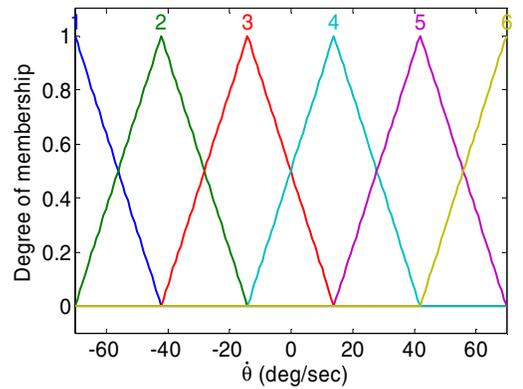
Figure 5. Membership functions for inverted pendulum problem
