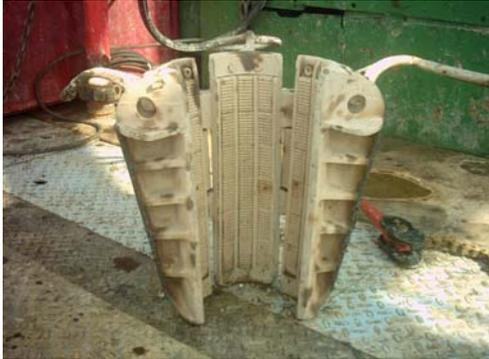
Figure 1: Slip is used to hanging the string
