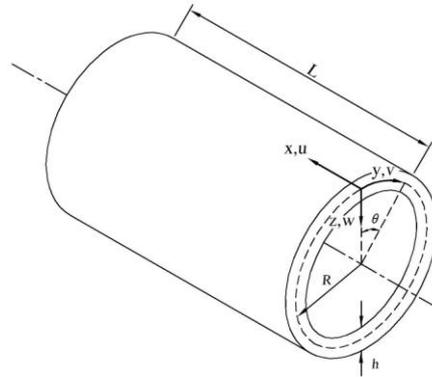
Figure 1 : Geometry and coordinate system of a cylindrical shell.
