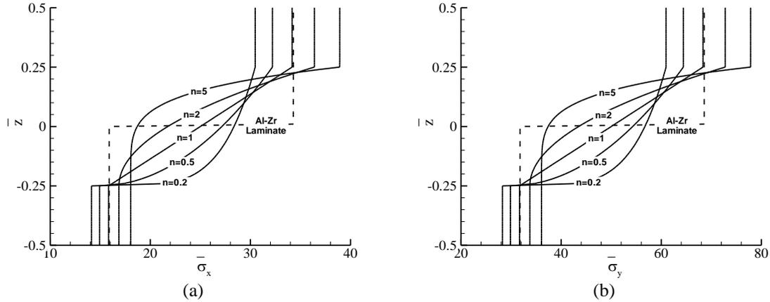
Figure 6 : Distributions of (a) longitudinal stress  $\bar{\sigma}_x$  and (b) circumferential stress  $\bar{\sigma}_y$  through the thickness of the FG cylindrical shell and the two-layer laminated cylinder at  $x=L/2$  due to the internal pressure  $P_z$ .
