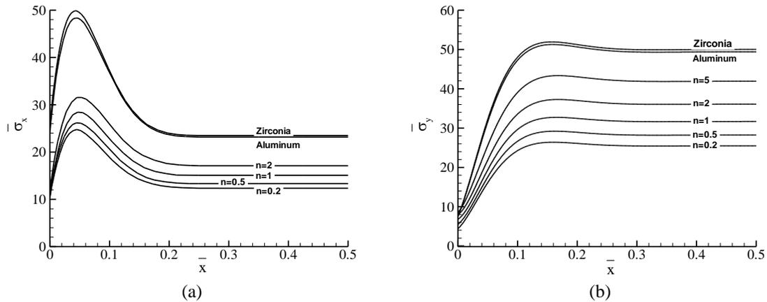
Figure 4 : Distributions of (a) longitudinal stress  $\bar{\sigma}_x$  and (b) circumferential stress  $\bar{\sigma}_y$  versus  $\bar{x}$  at the outer surface of the FG cylindrical shell due to the internal pressure  $P_z$ .
