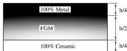
Figure 5 : Thickness of a cylinder made up of a FG layer at the mid-depth and two equal-thickness ceramic and metal layers at the inner and outer surfaces, respectively.
