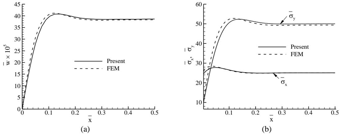
Figure 3 : Distributions of (a) deflection  $\bar{w}$  and (b) stresses  $\bar{\sigma}_x$  and  $\bar{\sigma}_y$  versus  $\bar{x}$  of the FG cylindrical shell ( $n=1$ ) due to internal pressure of  $P_z=1$  MPa.
