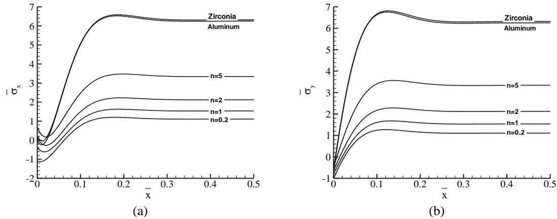
Figure 8 : Distributions of (a) longitudinal stress  $\bar{\sigma}_x$  and (b) circumferential stress  $\bar{\sigma}_y$  versus  $\bar{x}$  at the outer surface of the FG cylindrical shell due to the thermal loading.
