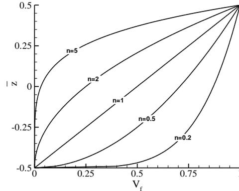
Figure 2 : Variation of the volume fraction  $V_f$  of the ceramic phase through the thickness of the FG cylindrical shell.
