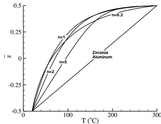
Figure 7 : Temperature profile through the thickness of the FG cylindrical shell.
