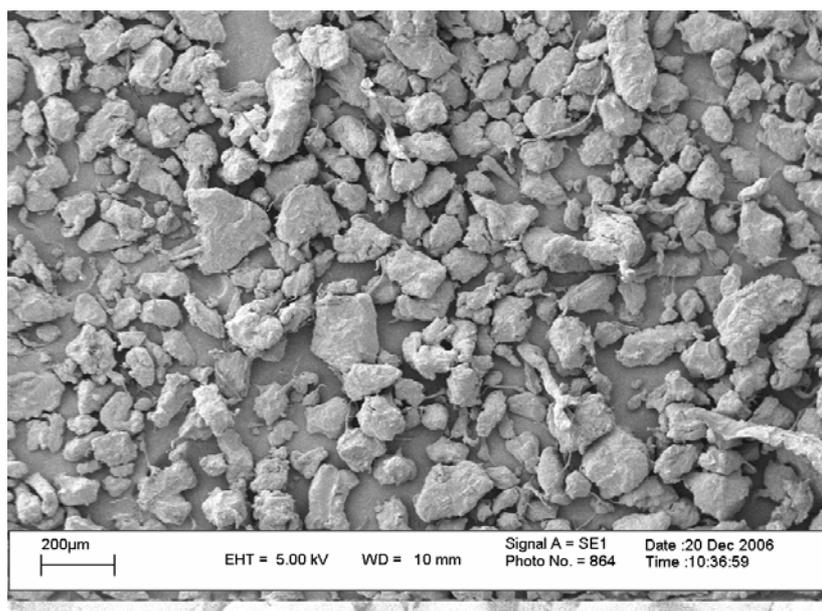
Figure 1: SEM micrograph of medium density polyethylene before milling
