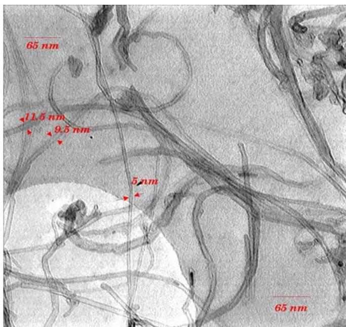
Figure 2: TEM micrograph of used carbon nanotube
