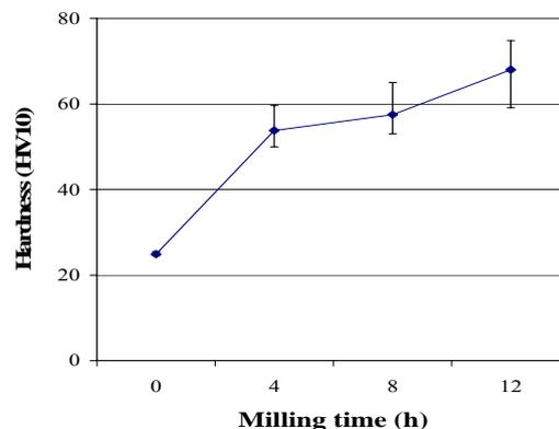
Figure 4. Hardness variation of Al-5%wt. Al<sub>2</sub>O<sub>3</sub> versus milling time.
