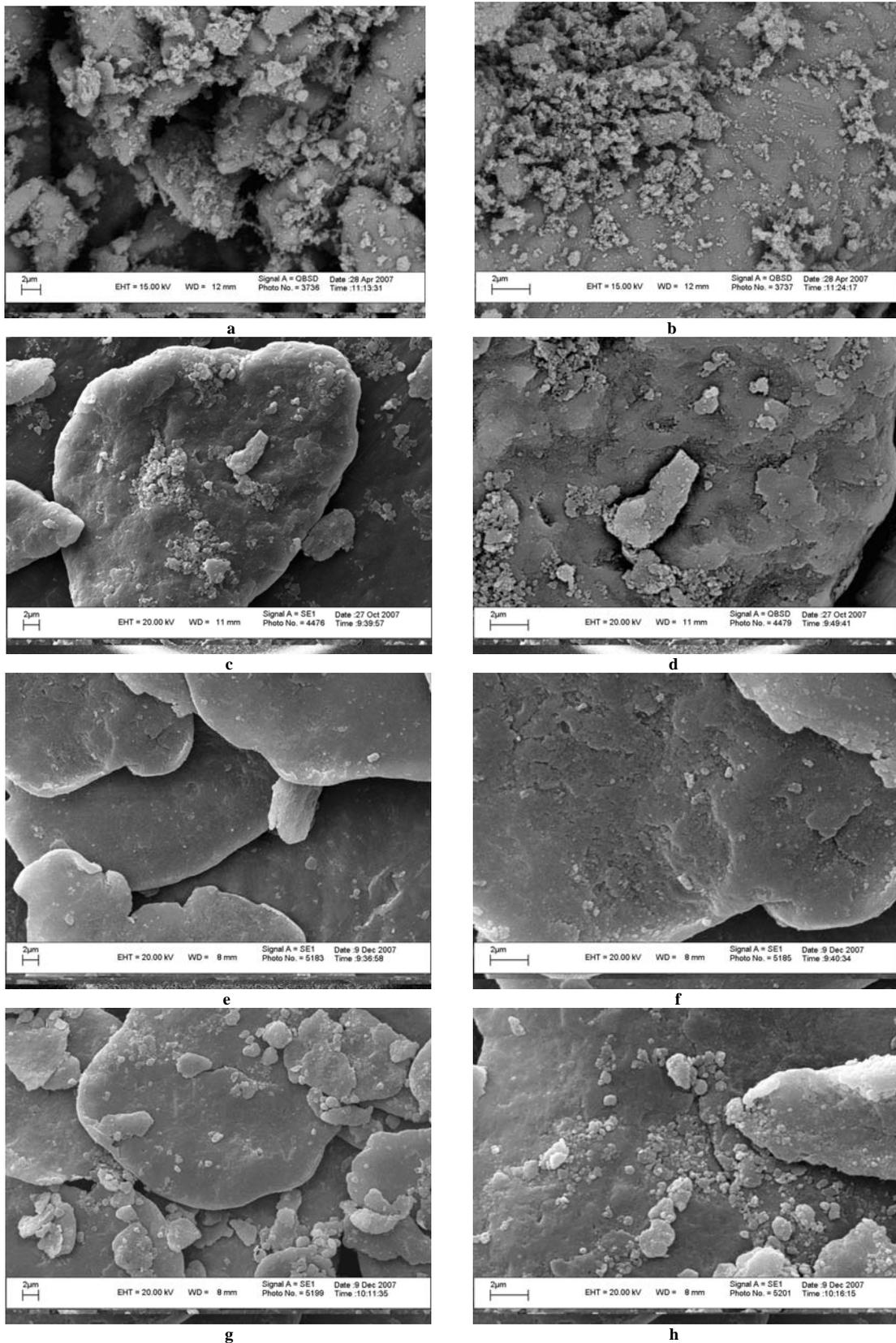
Figure 2. SEM Micrograph of Al-5 wt% Al<sub>2</sub>O<sub>3</sub> powder particles at various milling time: (a,b) 0h, (c,d) 4h, (e,f) 8h and (g,h) 12h.
