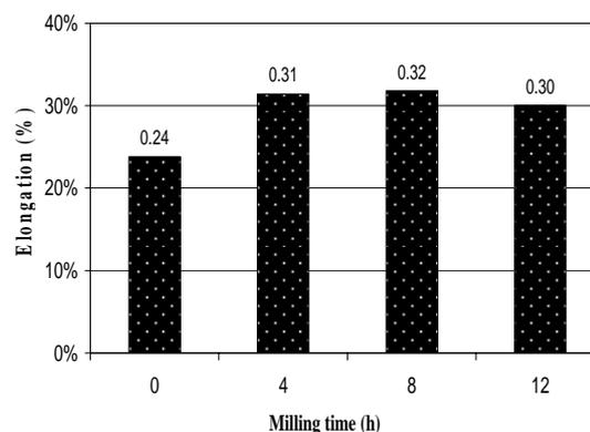
Figure 7. Elongation variation of the Al-5%wt. Al<sub>2</sub>O<sub>3</sub> versus milling time.
