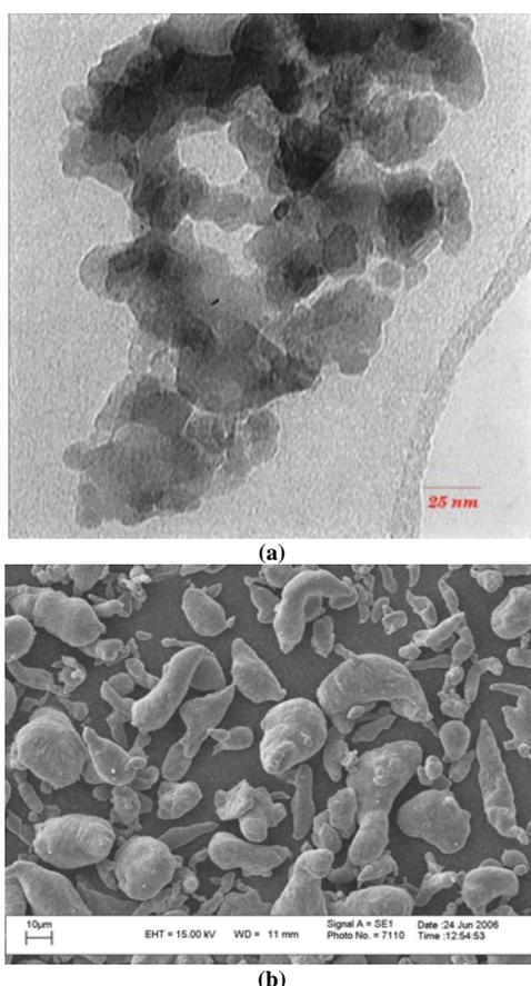
Figure 1. Initial used powders: (a)  $\alpha$ -alumina, (b) aluminum
