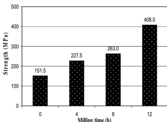
Figure 6. Strength variation of the Al-5%wt. Al<sub>2</sub>O<sub>3</sub> versus milling time.
