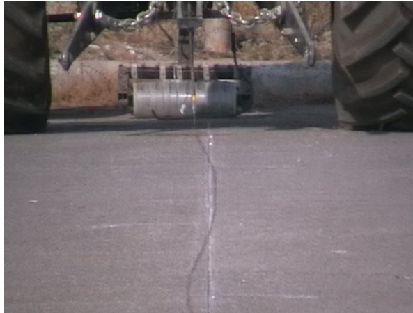
Fig7. Steering control system assembled on a MF285 tractor
