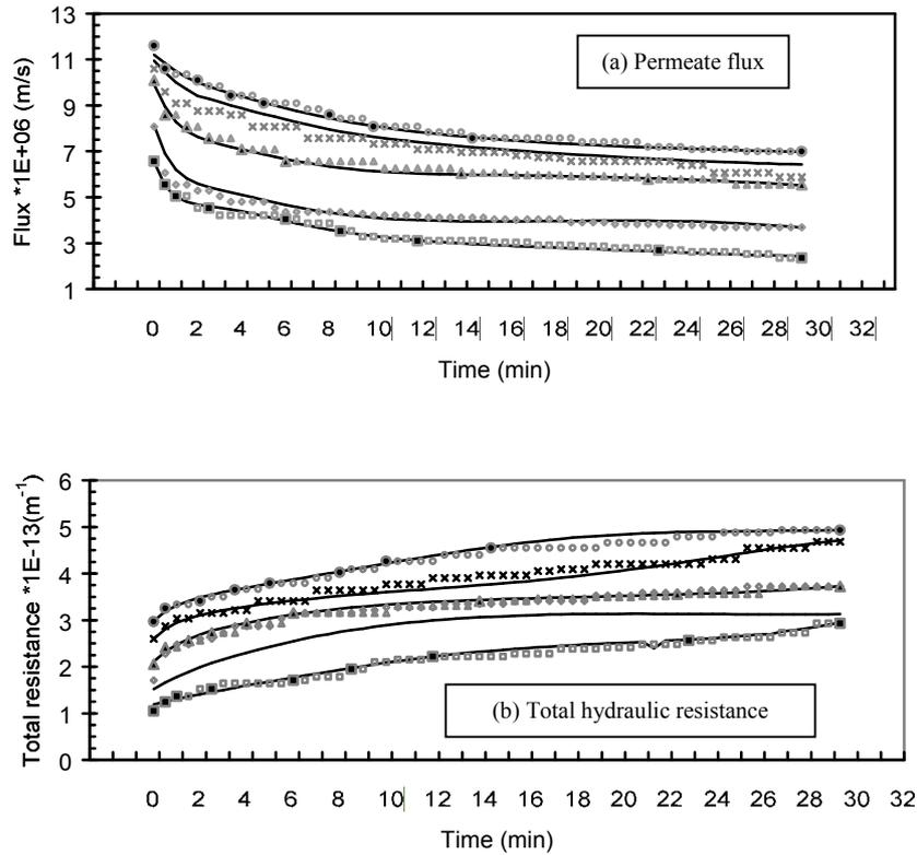
Fig. 1. Dynamic predictions of permeate flux and total hydraulic resistance during ultrafiltration of milk using training set (1). ANN used: 2/10/2. Training points are as solid symbols. Training points / Validation points / Querying points: 54/306/240. ( $\square$ , 50 kPa;  $\diamond$ , 100 kPa;  $\Delta$ , 150 kPa;  $\times$ , 200 kPa;  $\circ$ , 250 kPa; —, ANN)
