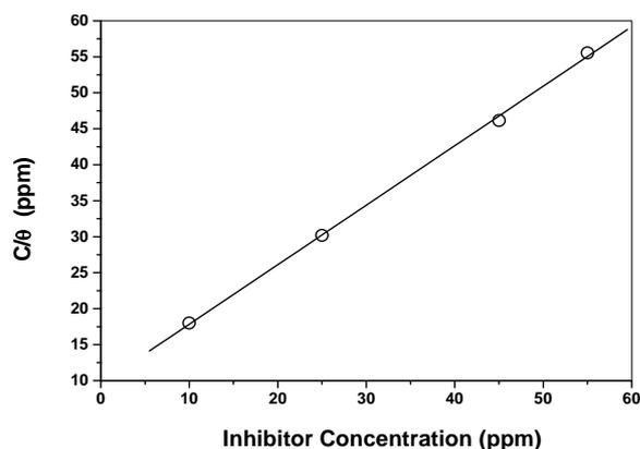
Fig. 3. Lungmuir isotherm curve fitting of corrosion data in  $\text{CO}_2$  environment at the presence of inhibitor.
