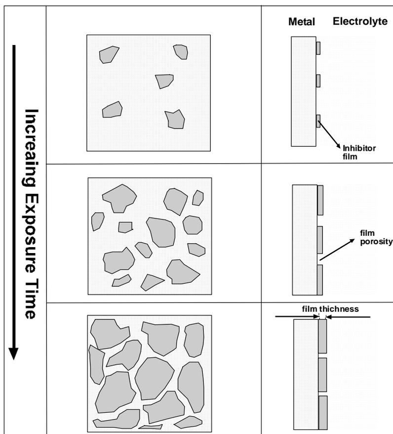
Fig. 10. Schematic illustration of inhibitor adsorption, polymerization and thickening on the electrode surface. The inhibitor is indicated by gray colonies.
