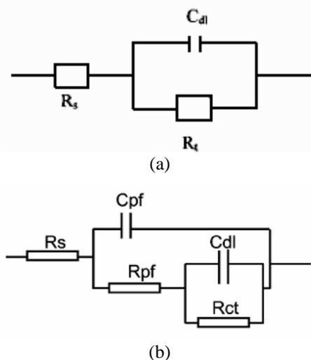
Fig. 6. Equivalent circuit used to represent the impedance results a) at the absence of corrosion inhibitor b) at the presence of corrosion inhibitor.
