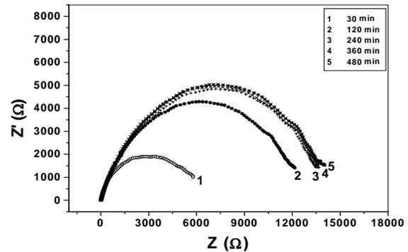
Fig. 9. EIS Nyquist plots for 40ppm inhibitor concentration at different exposure time.
