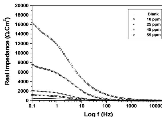
Fig. 7. Plots of real impedance vs.  $\log(f)$  for different concentrations of corrosion inhibitor.
