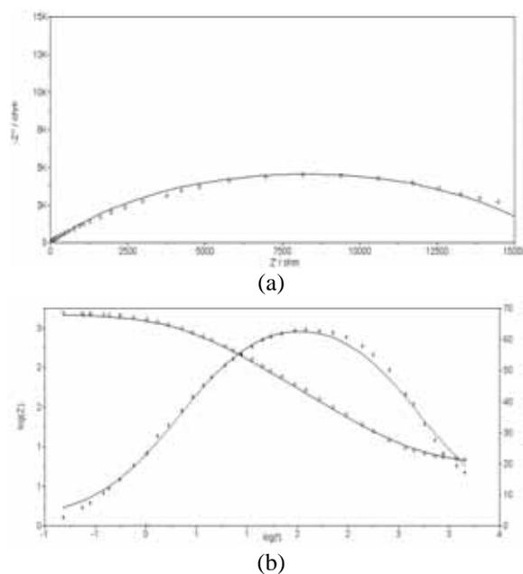
Fig. 4. EIS Nyquist (a) and Bode (b) plots for blank  $\text{CO}_2$  solution. Experimental data with (marker) and fitting model with (solid line) are shown.
