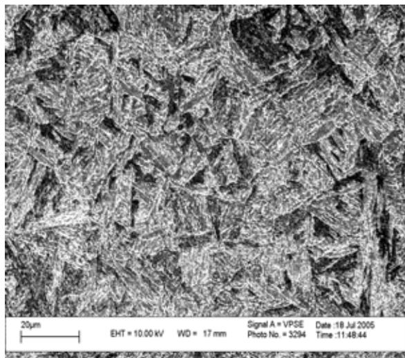
**Fig. 1.** SEM illustration of mild steel used in this work after etching in pickral.
