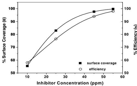
Fig. 8. Plots of inhibitor coverage and its efficiency as a function of inhibitor concentration.
