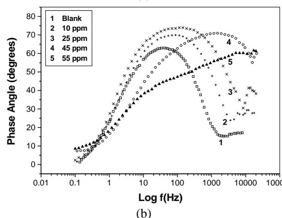
Fig. 5. a) EIS and Bode plots at different concentrations of corrosion inhibitor. In part (a) the Nyquist plot of working electrode in blank solution is highlighted.
