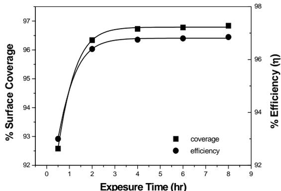
Fig. 11. Plots of inhibitor coverage and efficiency evolution for 40ppm inhibitor concentration.
