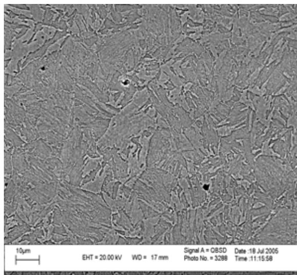
**Fig. 2.** Backscattered SEM image of mild steel used in this work after etching in pickral.
