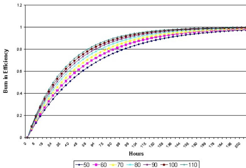
**Fig. 2:** The testing efficiency of burn in at constant temperature versus testing time
