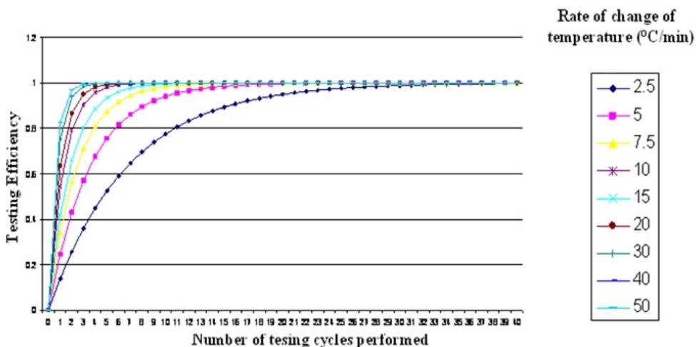
Fig. 7: The testing efficiency of thermal cycle screening for a temperature span of 140 degrees Celcius
