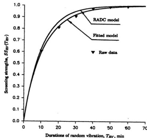
**Fig. 18:** A comparison of RADC model and fitted data for random vibration screen strength presented by (Kececioglu, *et al.*, 2002).
