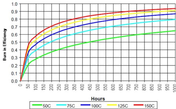
**Fig. 1:** The screening efficiency of constant temperature burn-in based on the Hughes model as reported in the literature
