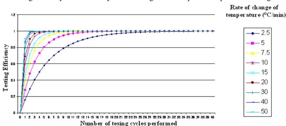
Fig. 9: The testing efficiency of thermal cycle screening for a temperature span of 180 degrees Celcius
