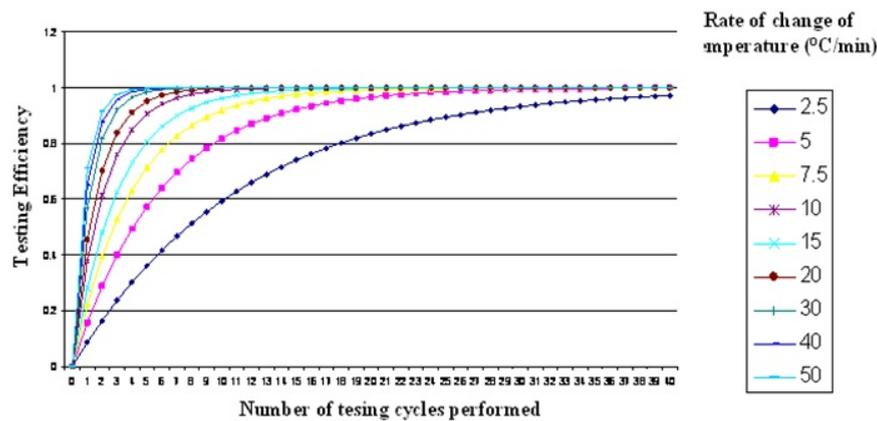
**Fig. 3:** The testing efficiency of thermal cycle screening for a temperature span of 60 degrees Celcius
