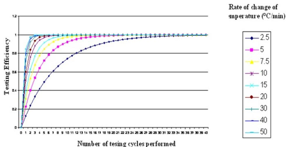
Fig. 6: The testing efficiency of thermal cycle screening for a temperature span of 120 degrees Celcius
