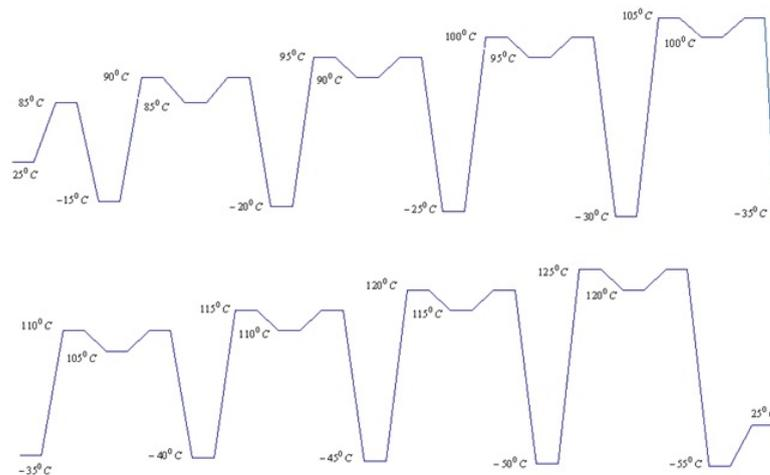
**Fig. 11:** The proposed destructive thermal cycle – the product is exposed to the test until it fails.
