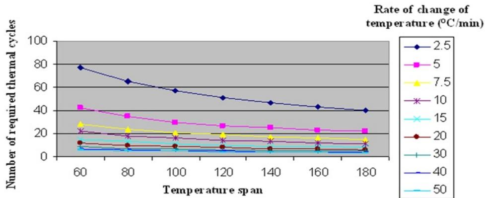
**Fig. 10:** The number of thermal cycles required to achieve a test efficiency of 0.999
