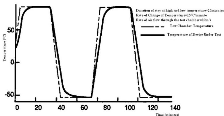
**Fig. 14:** A typical thermal cycling screen indicating the various parameters of interest
