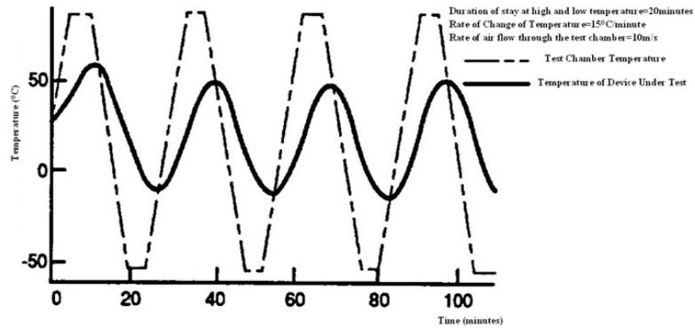
**Fig. 15:** A typical poorly designed thermal cycling screen indicating the inability of the device under test to follow the desired temperature
