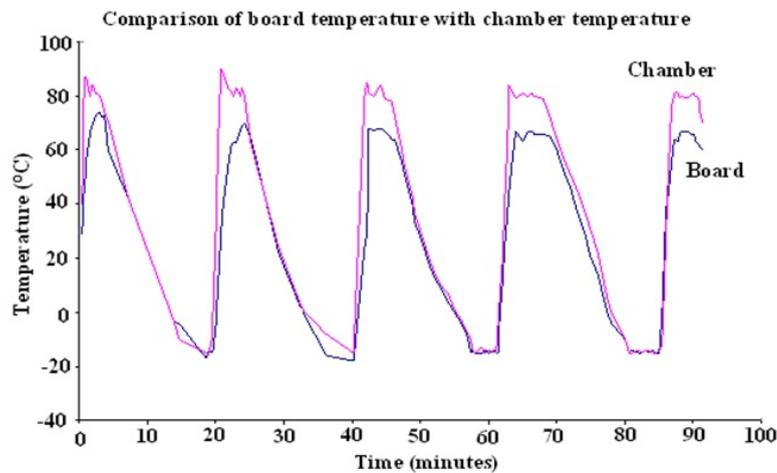
**Fig. 17:** An ESS thermal cycling screen using low to high rate of 25 degrees Celcius per minute and a high to low rate of 5 degrees Celcius per minute.
