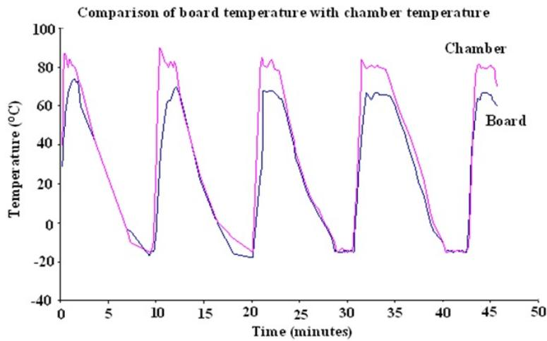
**Fig. 16:** An ESS thermal cycling screen using low to high rate of 50 degrees Celcius per minute and a high to low rate of 10 degrees Celcius per minute.
