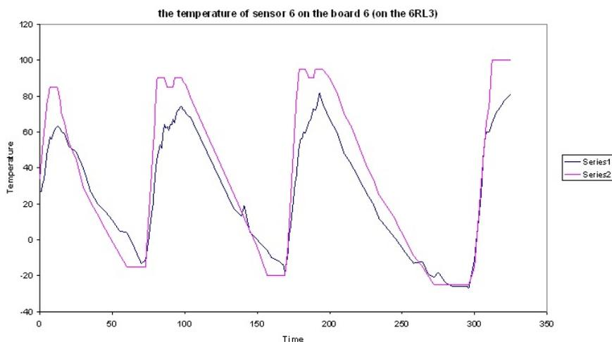
**Fig. 13:** The temperature profile of one of the boards of the electronic product under test compared with the expected temperature variations during HALT
