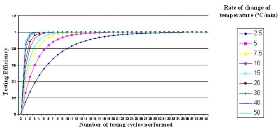
Fig. 8: The testing efficiency of thermal cycle screening for a temperature span of 160 degrees Celcius
