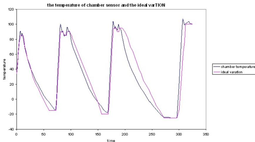
**Fig. 12:** The temperature profile of the chamber compared with the expected temperature variations indicating proper design of HALT
