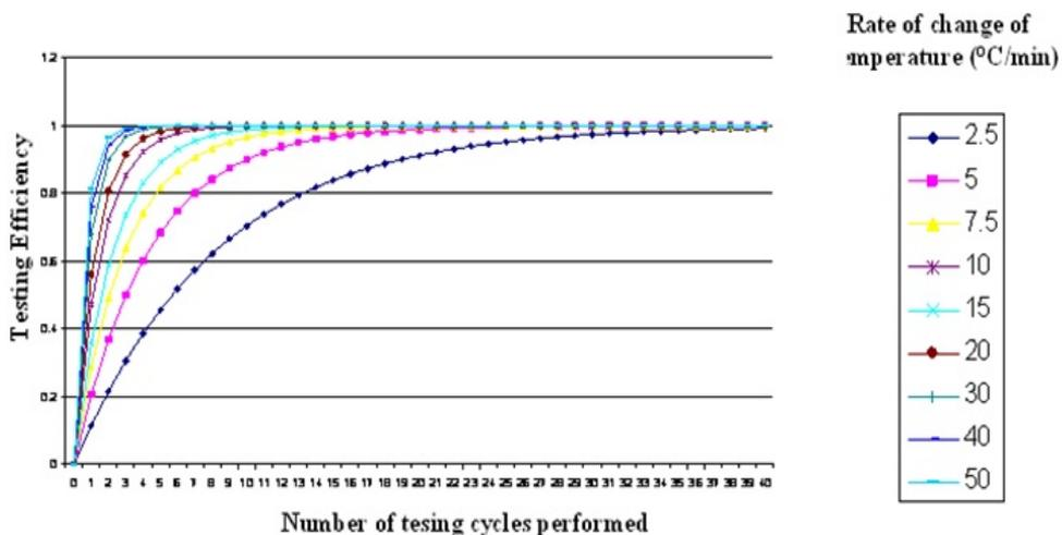
Fig. 5: The testing efficiency of thermal cycle screening for a temperature span of 100 degrees Celcius
