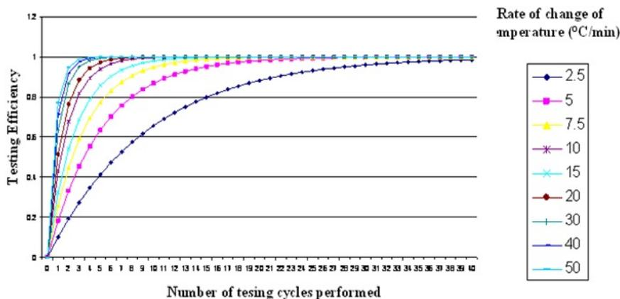
**Fig. 4:** The testing efficiency of thermal cycle screening for a temperature span of 80 degrees Celcius
