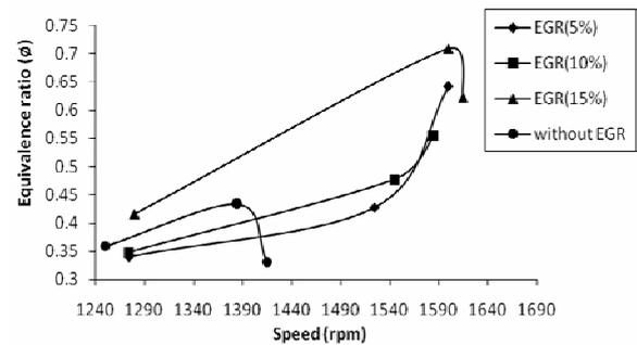
Figure 2: Variation of equivalence ratio with variation of engine speed in different EGR rates
