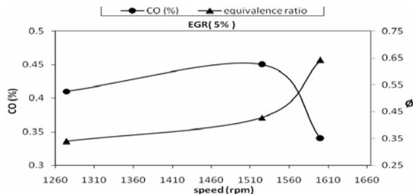
Figure 4: variations of equivalence ratio and CO emission with engine speed variation
