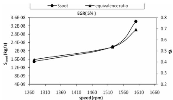
Figure 6: variations of equivalence ratio and soot emission with engine speed variation
