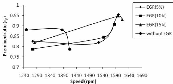
Figure 3: Variation of premixed ratio with variation of engine speed in different EGR rates
