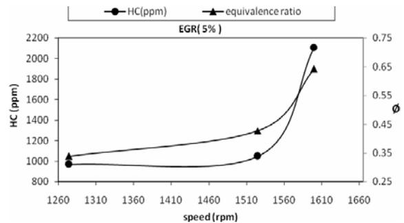
Figure 5: variations of equivalence ratio and HC emissions with engine speed variation
