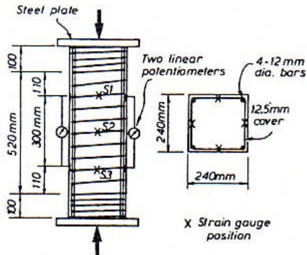
Figure 3. Geometrical specifications of samples [6]
