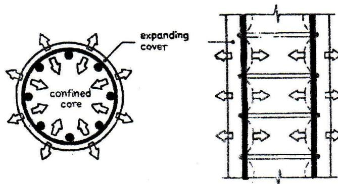
Figure 1. Mechanism of the cover collapsing
