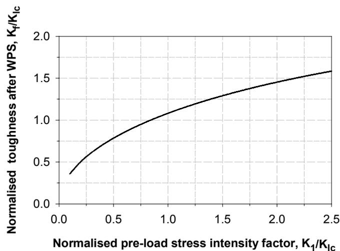
Fig. 3. Enhancement in toughness for A533B steel warm pre-stress at  $20^{\circ}\text{C}$ , fractured at  $-170^{\circ}\text{C}$
