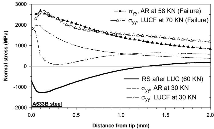
Fig. 2. Normal stress distribution for the as-received and warm pre-stressed conditions for A533B steel at  $-170^{\circ}\text{C}$
