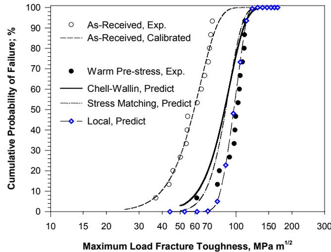
Fig. 4. Comparison of predictions of probability distribution following WPS based on "Global" and "Local" approaches for A533B steel at  $-170^{\circ}\text{C}$
