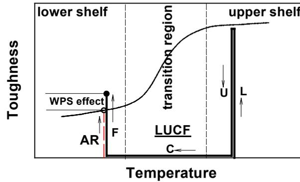
Fig. 1. Schematic description of WPS effect on cleavage fracture toughness
