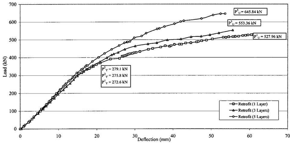
Fig. 10. Load versus deflection of retrofitted composite girders
