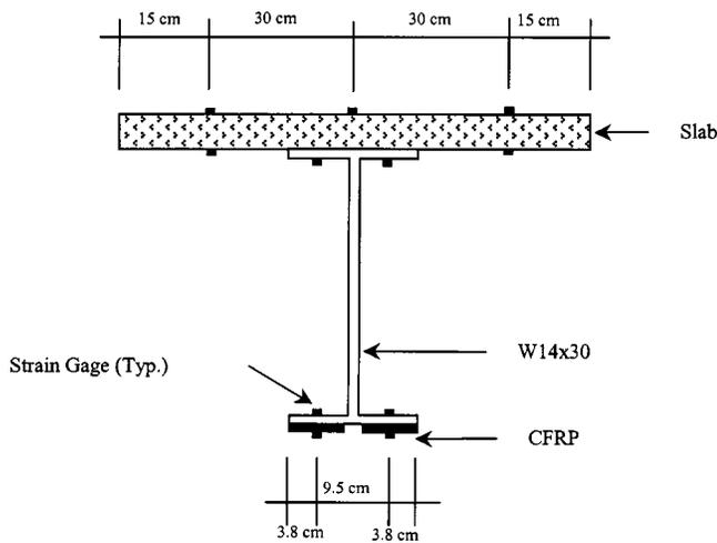
**Fig. 4.** Schematic of strain gage locations at midspan
