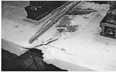
a) Concrete Crushing
