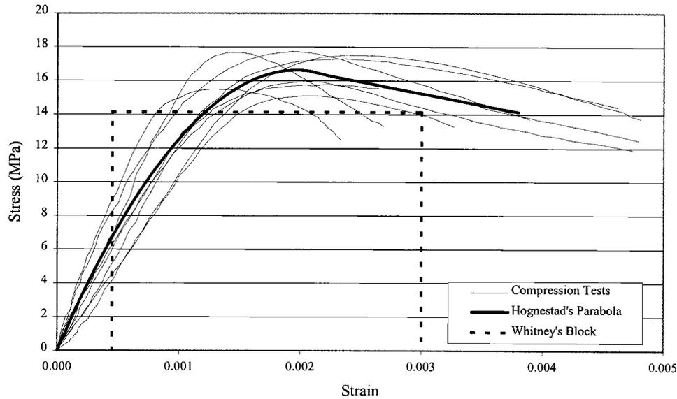
**Fig. 7.** Constitutive modeling of concrete
