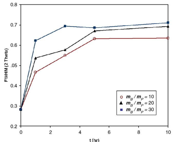
Fig. 4. The changes of the FWHM of (112) peak against milling time at constant ball to powder weight ratios.
