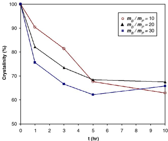
Fig. 6. Variation of crystallinity ( $X$ ) of (112) peak against milling time at constant ball to powder weight ratios ( $m_B/m_P$ ).
