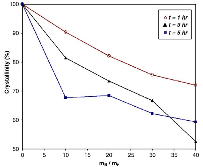
Fig. 7. Variation of crystallinity ( $X$ ) of (112) peak against ball to powder weight ratio at constant milling times ( $t$ ).
