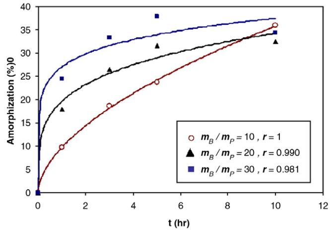
Fig. 8. Fitness of the proposed equation to the data of amorphization of chalcopyrite for different milling times and ball to powder weight ratios (data points from the present study).
