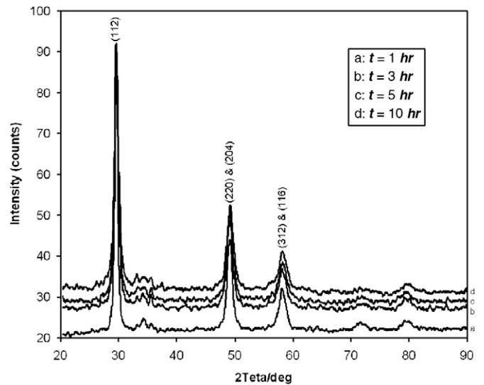
Fig. 3. X-ray diffraction patterns of mechanically activated chalcopyrite for ball to powder weight ratio of 10 and different milling time ( $t$ ).
