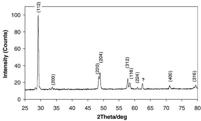
Fig. 1. X-ray diffraction pattern of natural chalcopyrite mineral.
