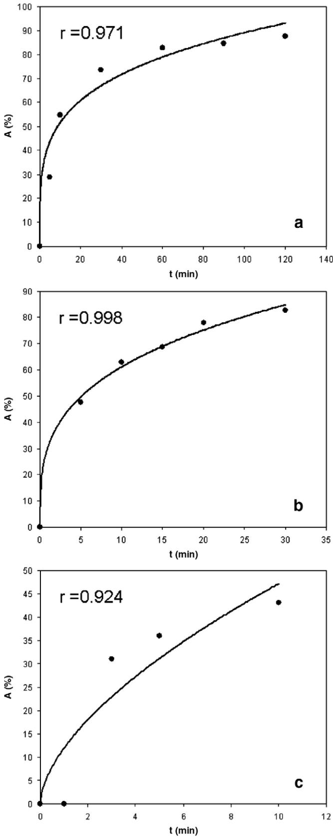
Fig. 10. Fitness of the proposed equation to the data of amorphization with the milling time for olivine in a) an attritor, b) a planetary and c) a nutating mill (data points extracted from Baláz et al., 2008).
