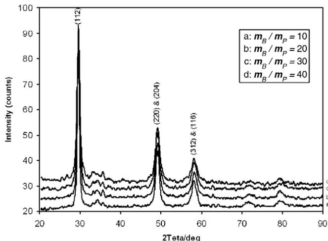
Fig. 2. X-ray diffraction patterns of mechanically activated chalcopyrite for 1 h milling time and different ball to powder weight ratios ( $m_B/m_P$ ).
