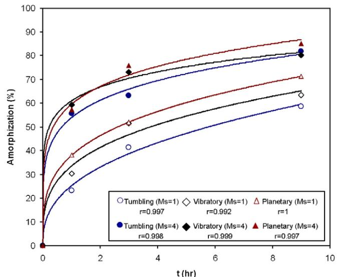
Fig. 9. Fitness of the proposed equation to the data of amorphization of hematite with the time of mechanical activation and milling media surface ( $m^2/kg$  of material) in different milling devices (data points from Poughahramani and Forssberg, 2006).
