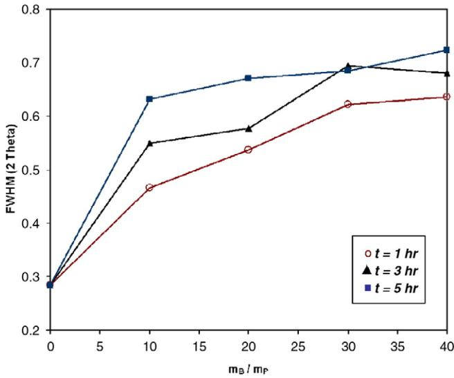
Fig. 5. The changes of the FWHM of (112) peak against ball to powder weight ratio for constant milling times.
