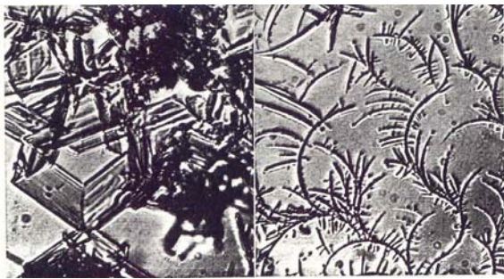
Figure 1. Initial microstructure of 2024 Al alloy versus direct Extrusion.
