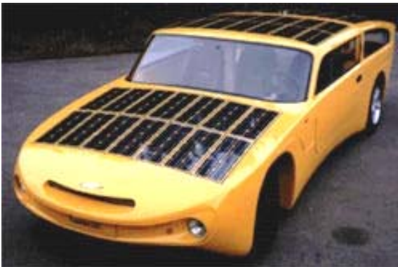
Figure 2: Toria, an electric vehicle equipped with solar cells
