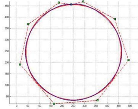
Fig. 2. Control polygon and approximated B-spline curve of degree 3 over 400 data points
