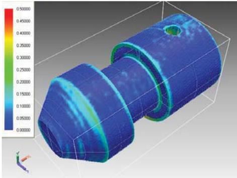
Fig. 11. Deviation of cloud point from original CAD model
