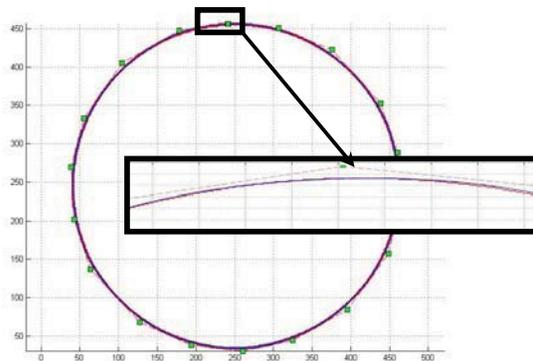
Fig. 3. Closed B-spline curve of degree 3.
