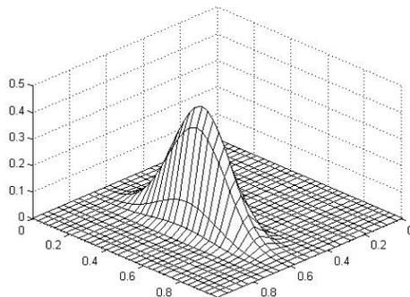
Fig. 4. Basis function for B-spline surface which is product of two one-dimensional B-spline basis function
