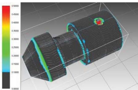
Fig. 12. Deviation of reconstructed model from original CAD model with acceptable tolerance (0. 1mm).
