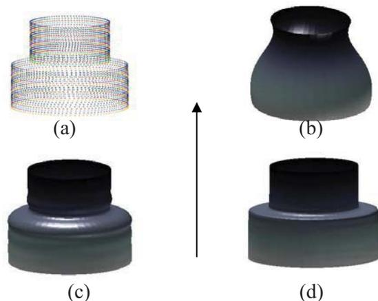
Fig. 6. Influence of increasing the number of control points on sharp edges reconstruction
