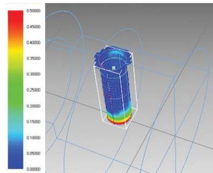
Fig. 14. Deviation of reconstructed model from original CAD model.
