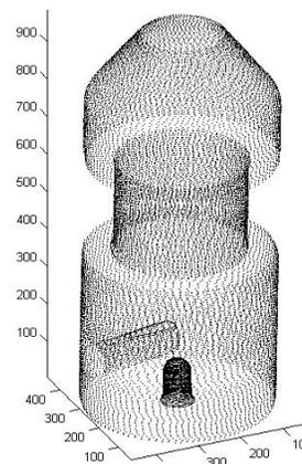
Fig. 10. Extracted cloud point from 2D images
