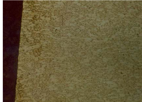
Figure 15: grain features in machined surface edge and non-machined surface
