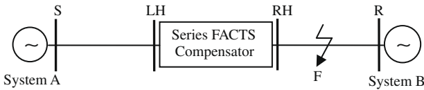
Fig. 3. One-line diagram of a series FACTS compensated transmission line.
