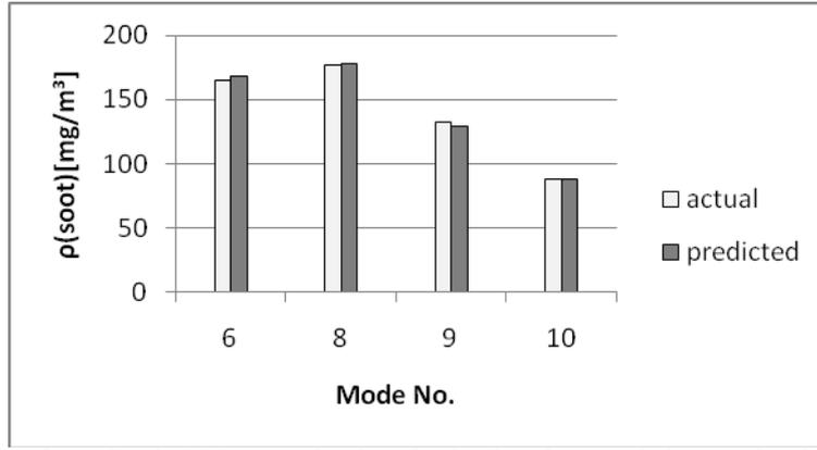
Fig.7. Comparison of actual and ANN approach values for density of soot emission test data(high density modes)
