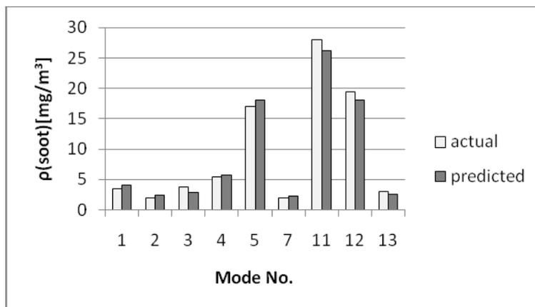
Fig.6. Comparison of actual and ANN approach values for density of soot emission test data(low and average density modes)
