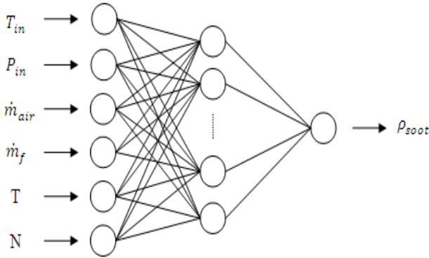
Fig.4. ANN architecture with 25 neurons in a single hidden-layer
