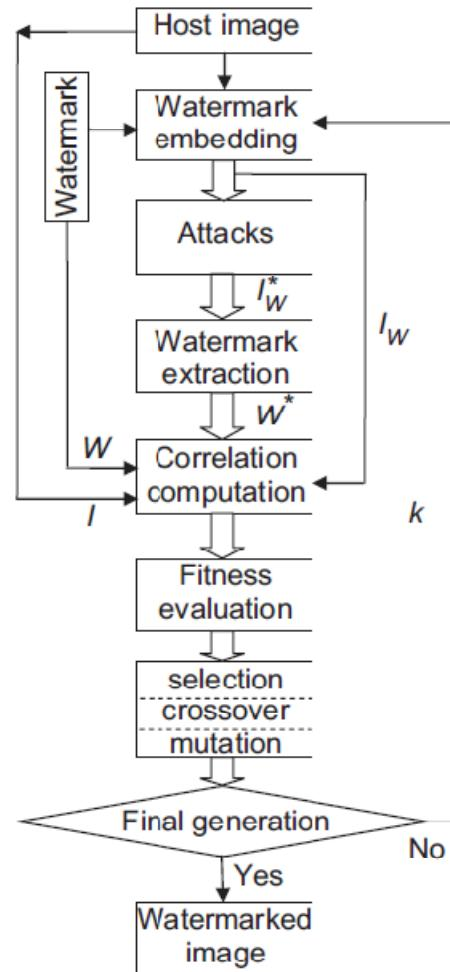
**Figure 1. Watermarking algorithm block diagram.**
