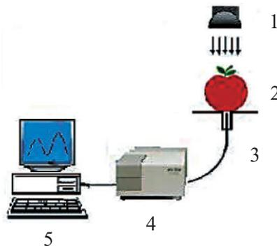
FIG. 1. VIS/NIRS EXPERIMENTAL INSTRUMENT SET UP FOR TRANSMISSION MODE (V): (1) LIGHT SOURCE; (2) SAMPLE; (3) FIBER OPTIC; (4) SPECTROMETER; AND (5) COMPUTER
