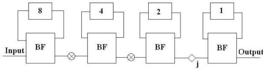
Fig.2. 16-point R2SDF pipeline FFT processor.
