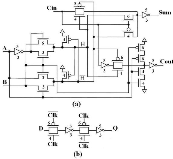
Fig.4. (a) Selected 1bit-full adder circuit. (b) Selected d-flip-flop circuit.
