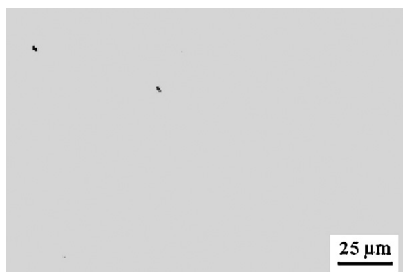
Fig. 3. Microstructure of CK45 steel sample before heat treatment and after more polishing (without etching). The spots which exist on the surface show a decrease in comparison with Fig. 2.
