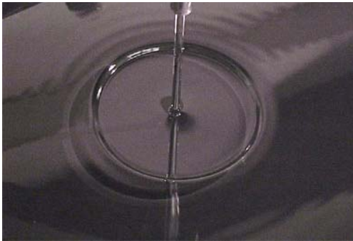
Figure 1: The circular hydraulic jump (Bush and Aristoff, 2003).
