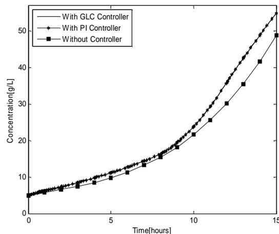
Fig 8. Closed loop response of cell concentration, GLC method (line), PI controller (line-star), without controller (line- square)
