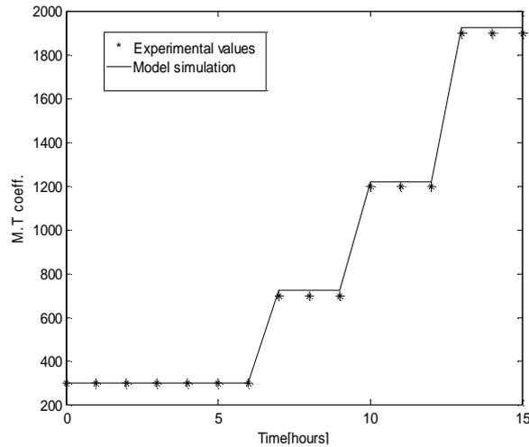
Fig 5. Experimental data [7] and model simulation for the  $K_La$
