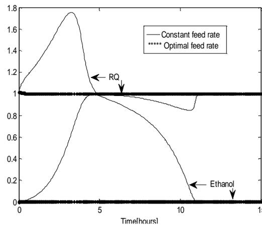
Fig 3. Ethanol concentration and RQ with constant and optimal feed rate
