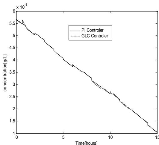
Fig 7. Closed loop response of oxygen concentration, GLC method (dash line), PI controller (line)
