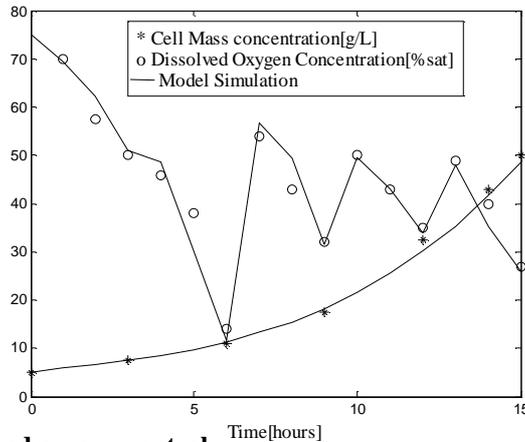
Fig 6. Experimental data [7] and model simulation for the biomass and oxygen concentration
