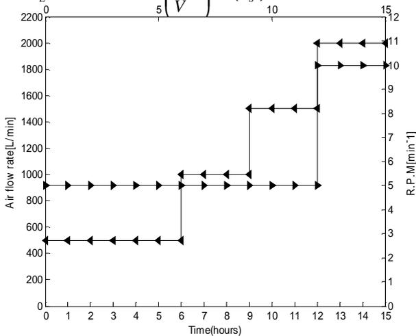
Fig 4. Experimental data of the air flow and stirrer speed rates[7]
