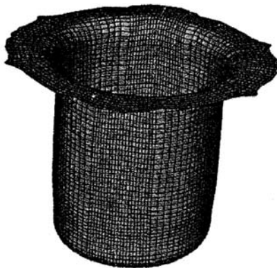
Fig. 20. A successful produced cup with drawing ratio 3.67, N=84
