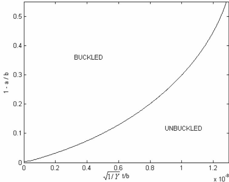
Figure 7. Wrinkling rea for laminated, St-St, Al-Al, St-Al
