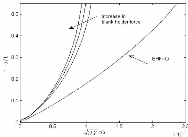
Figure 8. The Effect of changing blankholder force on onset of wrinkling
