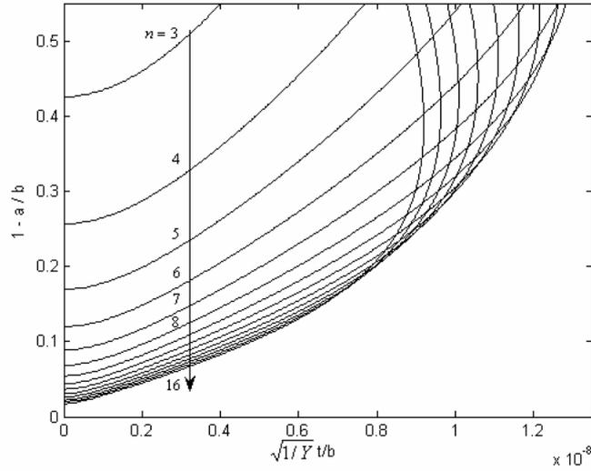
Figure 5. Onset of wrinkling for different  $n$ 's.
