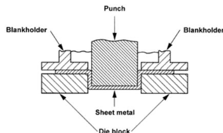
Figure 1. Deep drawing process with cylindrical punch
