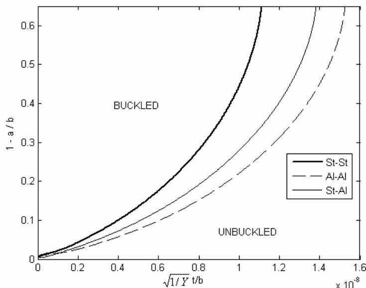
Figure 8. Onset of wrinkling of laminated, St-St, Al-Al and St-Al
