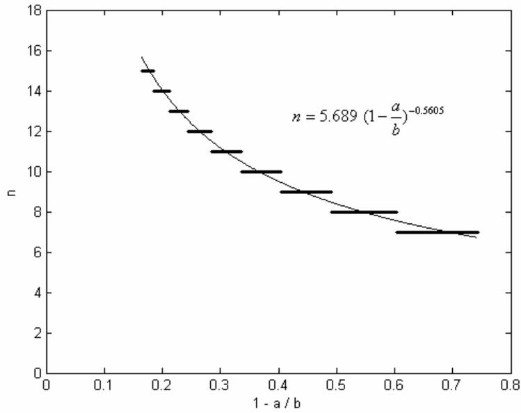
Figure 6. Onset of wrinkling for laminated, St-St, Al-Al, St-Al
