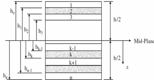
Figure 4. The coordinate of laminated plates
