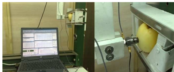
Fig. 1: General view of the pendulum device for measuring impact force and impact velocity of the apple fruit
