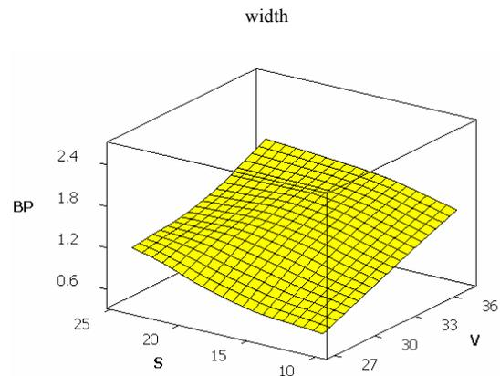
Fig. 8 The effects of welding speed and voltage on weld penetration
