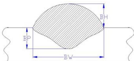
Fig. 2 Weld Bead Geometry Characteristics
