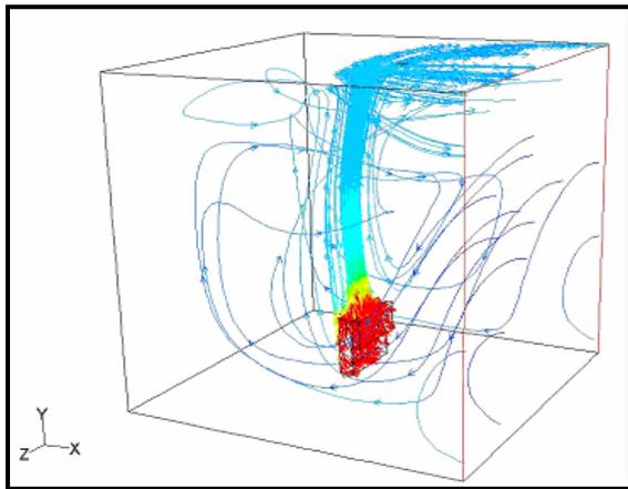
Figure13 Path of the air particles because of the produced movement due to temperature difference in the room with three walls
