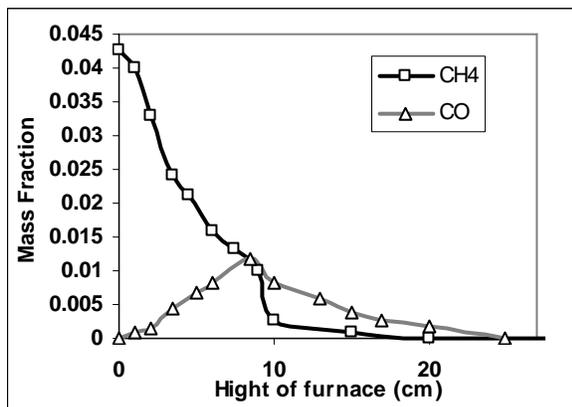
Figure 4 Variations of methane and carbon dioxide mass fraction with respect to furnace height
