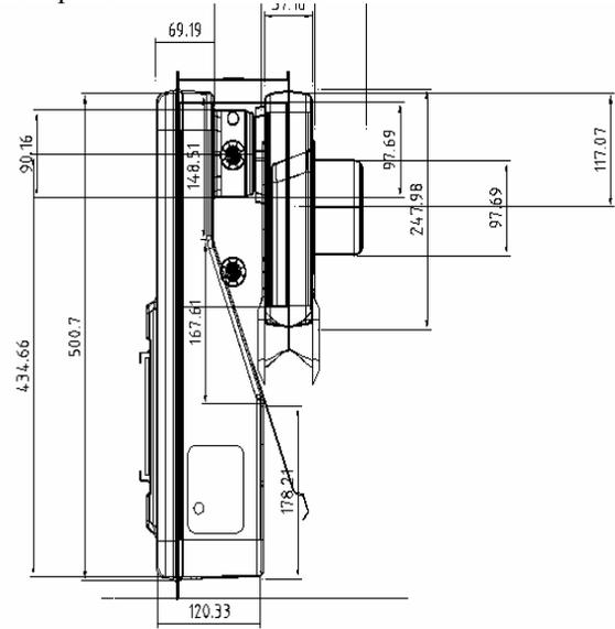
Figure1 Side view of the furnace of the gas-burner
