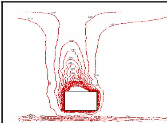
Figure 9 Temperature distribution around the gas-burner with radiation effects
