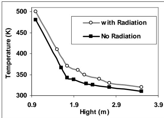
Figure 7 Temperature distribution produced by gas-burner with respect to height, in the centre of the room, in two cases of with and without radiation effects
