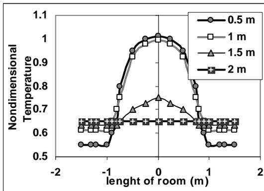
Figure12 Temperature distribution in the room with four lateral walls in four different heights with respect to room length
