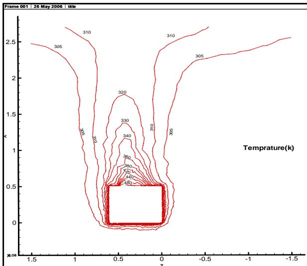
Figure 8 Temperature distribution around the gas-burner without radiation effects
