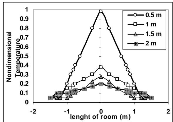
Figure 11 Temperature distribution in the room with three lateral walls in four different heights with respect to room length
