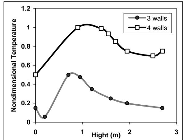
Figure 10 Non-dimensional temperature distribution with respect to height in the centre of the room, in two cases of three and four walls
