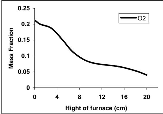
Figure 6 Variations of oxygen mass fraction with respect to furnace height
