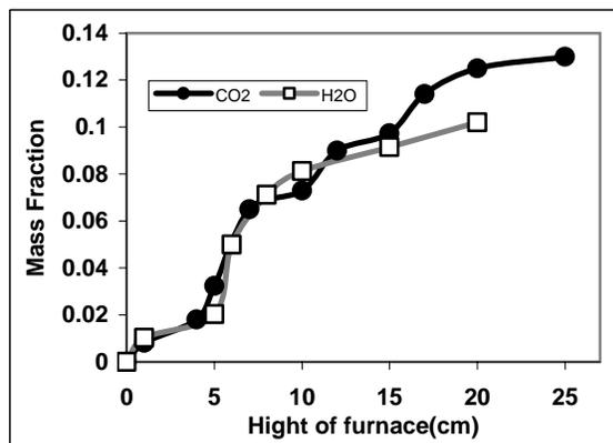
Figure 5 Variations of water and carbon dioxide mass fraction with respect to furnace height
