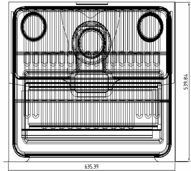
Figure 2 Front view of the furnace of the gas-burner
