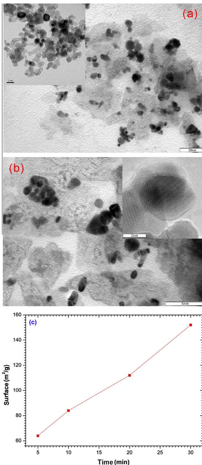
Fig. 4. HRTEM images of the prepared CdS: (a) stirring, 30 min; (b) sonication, 30 min and (c) surface area versus time.
