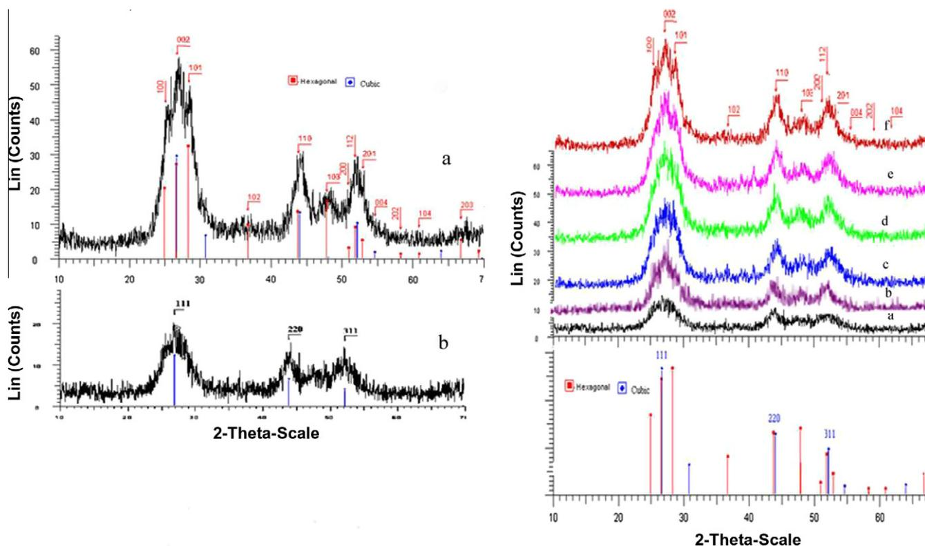
**Fig. 2.** X-ray diffraction patterns of the prepared CdS in: (a) sonication, 45 min; (b) stirring, 30 min. *Insert:* X-ray diffraction patterns of the prepared CdS in (a) stirring, 30 min; (b) homogenizer at 11,000 rpm, 30 min; (c) sonication, 5 min; (d) sonication, 15 min; (e) sonication, 30 min and (f) sonication, 45 min.
