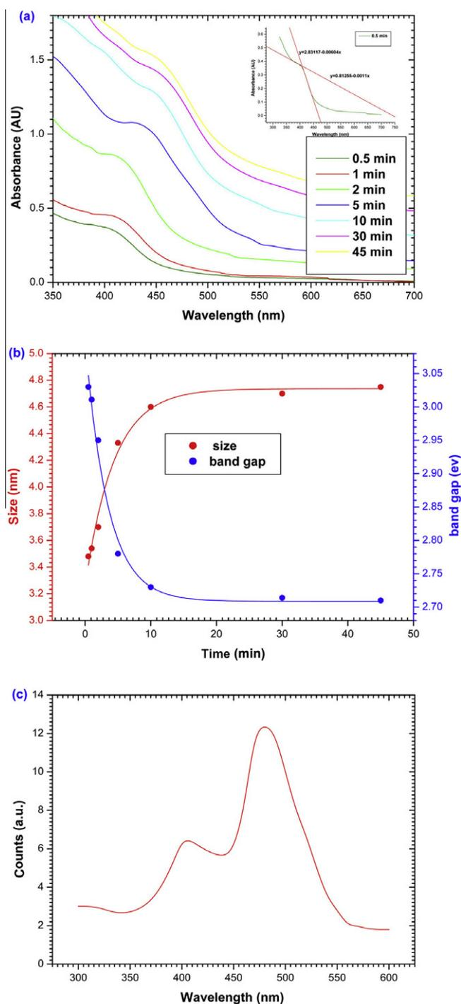
**Fig. 7.** (a) UV-visible spectra of samples at different interval times, (b) time of sonication on the optical size and band-gap of nano-particles, (c) photoluminescence spectrum of CdS nano-particle.
