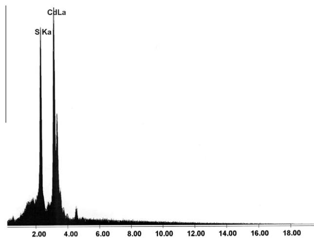
Fig. 5. EDAX measurement of the prepared CdS nano-crystals.
