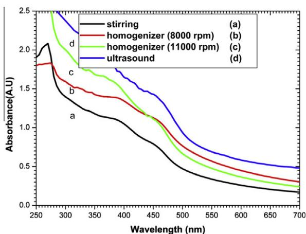
Fig. 8. UV-visible spectra of samples prepared in 30 min by different methods.
