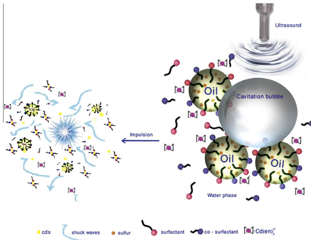
**Fig. 3.** Proposed reaction mechanism.
