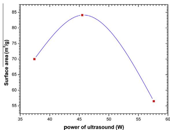
Fig. 6. Effect of intensity of ultrasound on nano-particles in 10 min of sonication.
