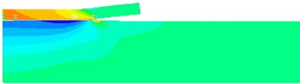
b) Figure 5: Typical simulation results of the temperature and structural deformation of the splat: a) temperature distribution; b) stress distribution
