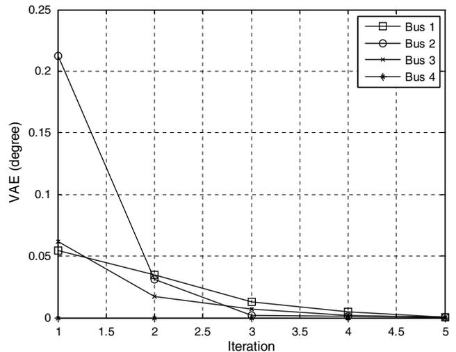
Fig. 2. Voltage angle errors at different iterations for 4-bus test system.
