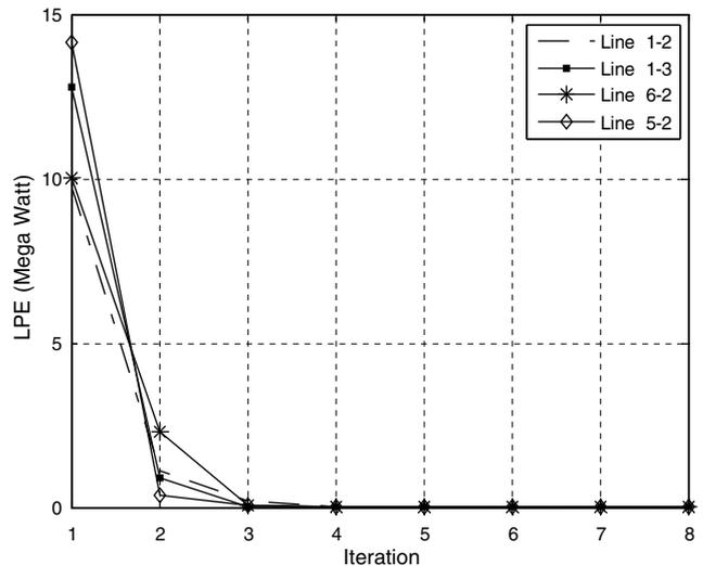
Fig. 7. LPEs for a few lines at different iterations, IEEE 30-bus test system.
