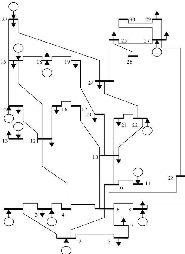
Fig. 5. Single line diagram of IEEE 30 buses test system.
