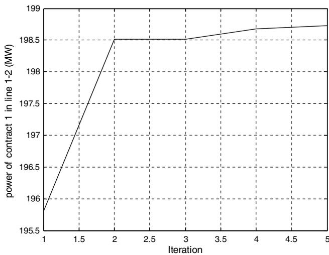
Fig. 4. Power flow of contract 1 in line 1–2 for 4-bus test system.
