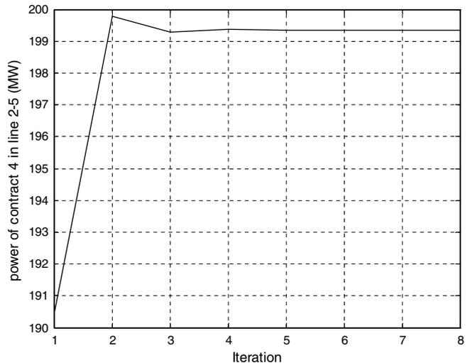
Fig. 8. Power flow of contract 4 in line 2-5, IEEE 30-bus test system.
