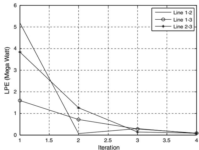
Fig. 3. Line power errors at different iterations for 4-bus test system.
