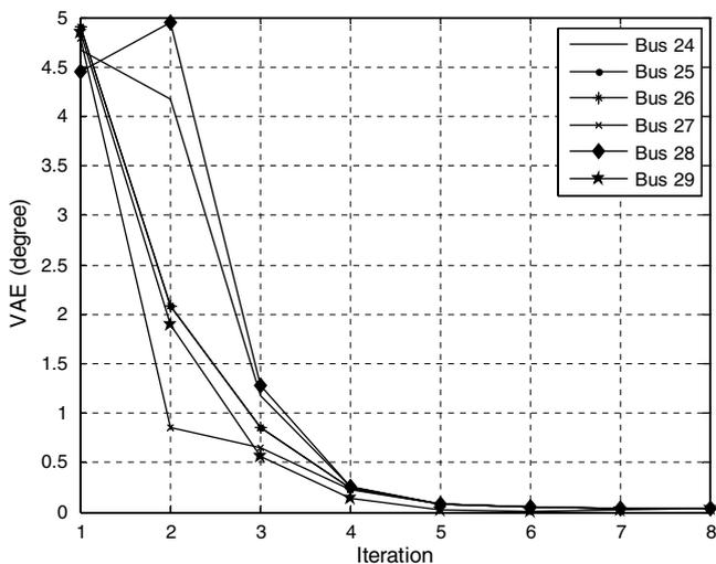
Fig. 6. VAEs for a few buses at different iterations, IEEE 30-bus test system.
