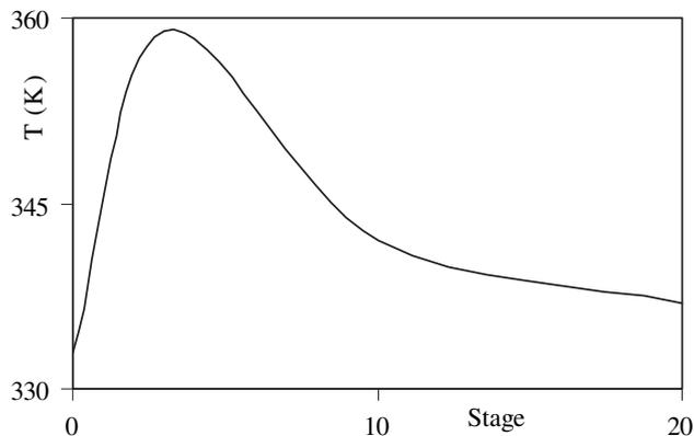
Fig. 1. Temperature profile across the amine absorption column.
