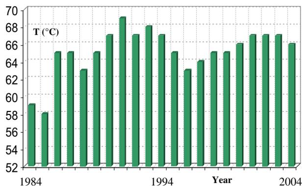
Fig. 2. Sour gas temperature increase during period of 1984–2004.
