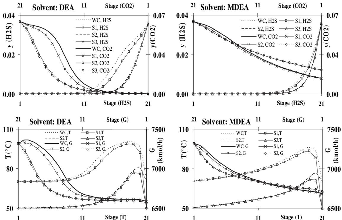
Fig. 10. Temperature, gas flow rate and vapor compositions distributions across the contactor using HYSYS program for various solvents with different cooling scenarios.
