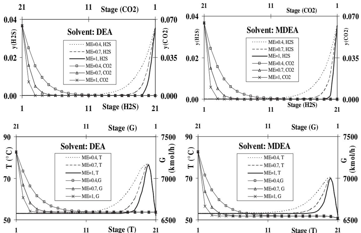
Fig. 5. Temperature, gas flow rate and vapor compositions distributions for contactor using Aspen at normal operating conditions for various efficiencies and different solvents.
