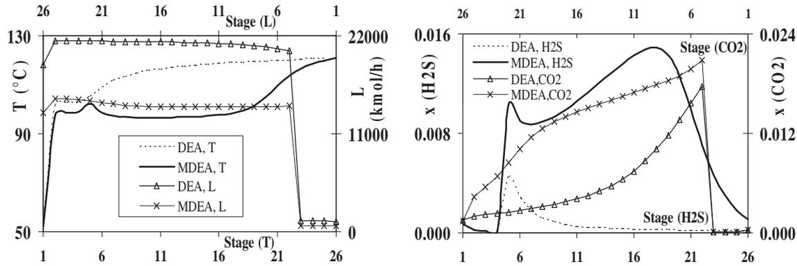
Fig. 7. Temperature, liquid flow rate and compositions distributions for stripper using HYSYS at normal operating conditions with different solvents.
