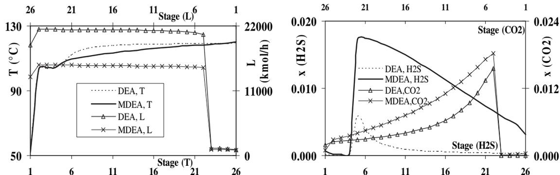
Fig. 8. Temperature, liquid flow rate and compositions distributions for stripper using Aspen at normal operating conditions with different solvents.
