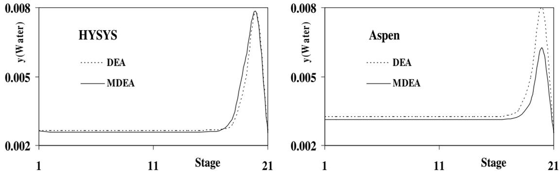
Fig. 6. Gas phase water mole fraction distributions across contactor using HYSYS and Aspen at normal operating conditions for various solvents at unit efficiencies.
