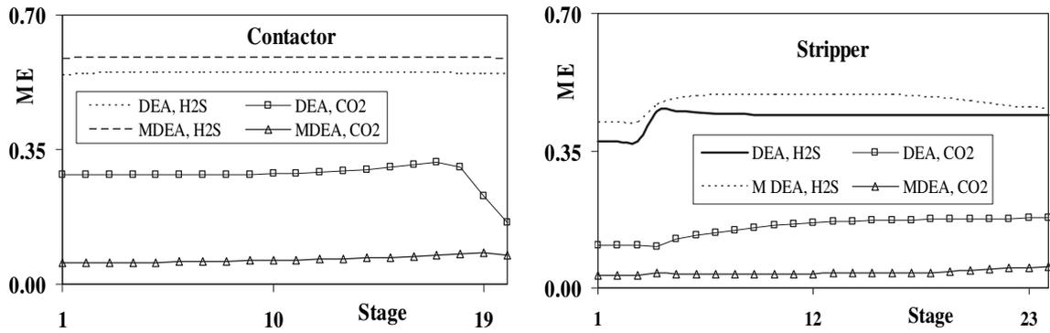
Fig. 9. Variation of automatically computed efficiencies across contactor and stripper.
