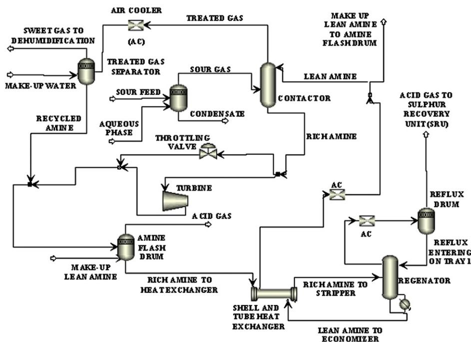
Fig. 3. Simplified schematic diagram of a Khangiran refinery GTU train.
