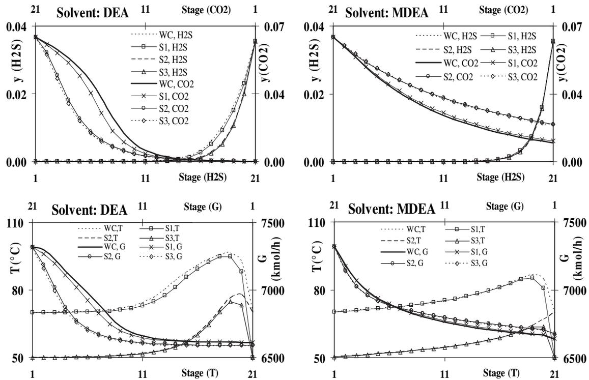
Fig. 11. Temperature, gas flow rate and vapor compositions distributions across the contactor using Aspen program for various solvents with different cooling scenarios.
