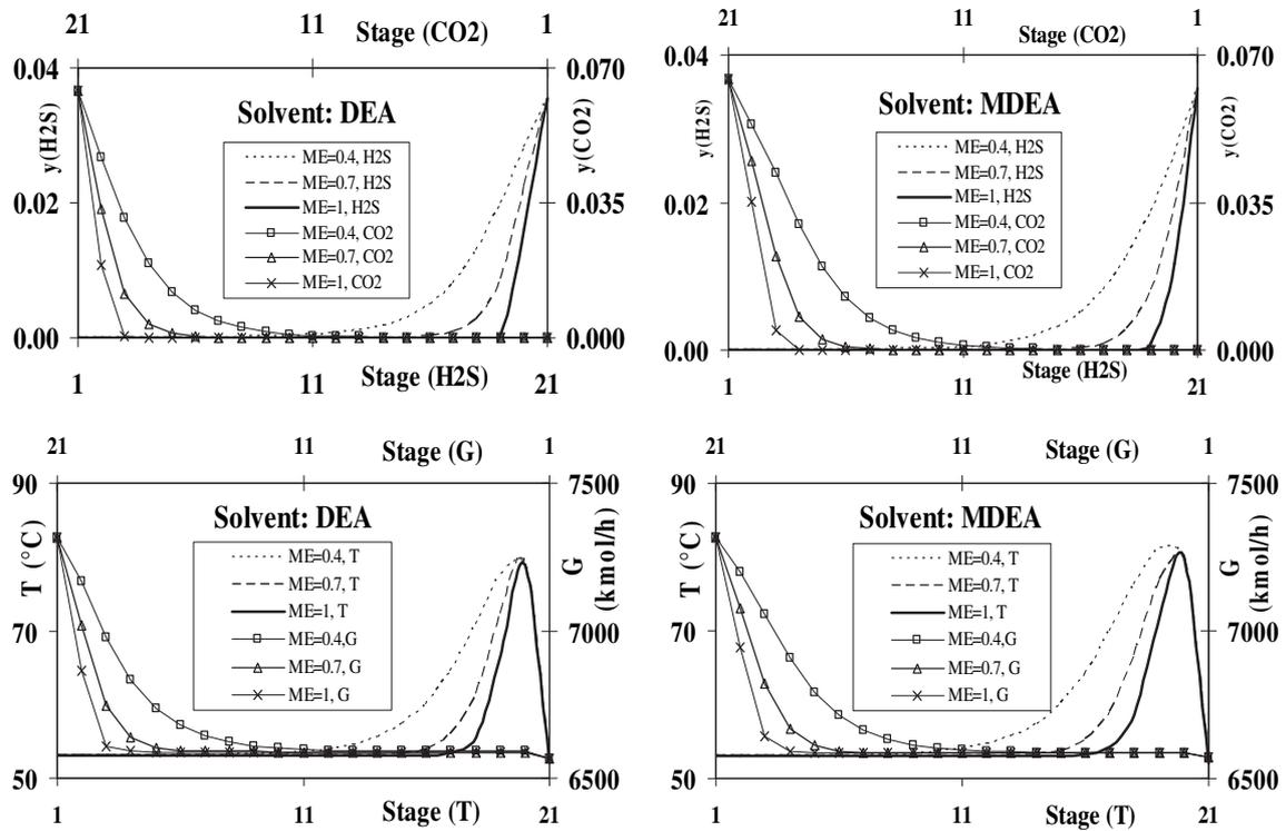
Fig. 4. Temperature, gas flow rate and vapor compositions distributions for contactor using HYSYS at normal operating conditions for various efficiencies and different solvents.
