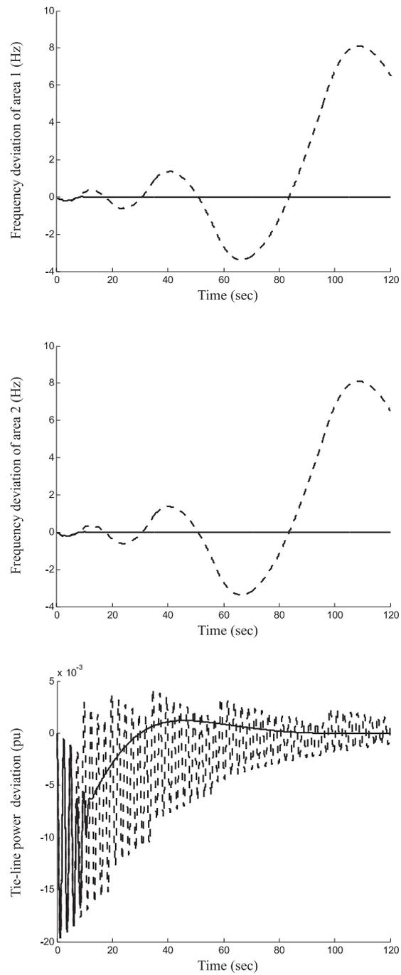
**Fig. 8** Dynamic responses for two different control strategies for case 3:  $\Delta P_{D1} = 1\%$ ,  $\Delta P_{D2} = 3\%$ . Fixed gain integral controller (---); Proposed controller (—).
