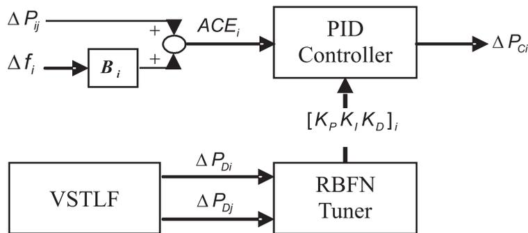
Fig. 2 The proposed controller block diagram.
