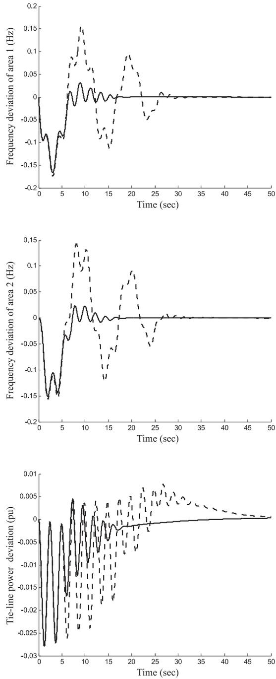
**Fig. 7** Dynamic responses for two different control strategies for case 2:  $\Delta P_{D1} = 3\%$ ,  $\Delta P_{D2} = 0$ . Fixed gain integral controller (---); Proposed controller (—).
