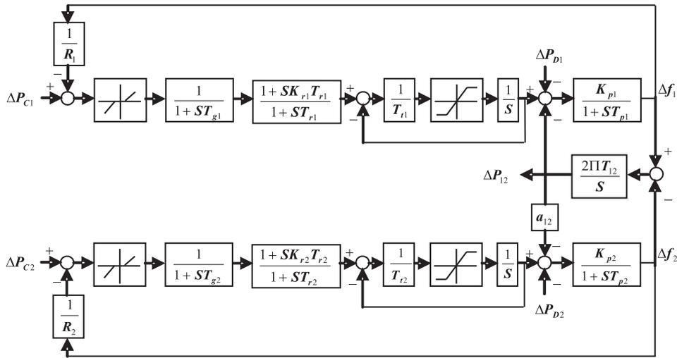
Fig. 1 The sample two-area power system block diagram.
