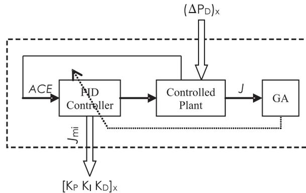
**Fig. 3** The offline application of GA in order to obtain the optimum PID constants.
