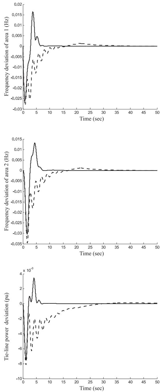
**Fig. 6** Dynamic responses for two different control strategies for case 1:  $\Delta P_{D1} = 1\%$ ,  $\Delta P_{D2} = 0$ . Fixed gain integral controller (---); Proposed controller (—).
