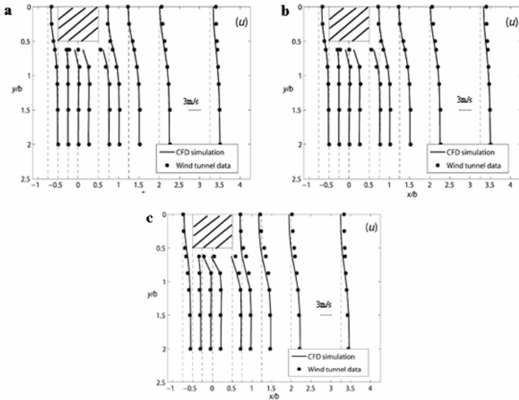
**Figure 4:** Comparison between wind tunnel data with simulation results by RKE. Vertical cross section along centerline of building on (a), on horizontal plane at  $z = 1.25b$  on (c) and on horizontal plane at  $z = 0.125b$  on (e)
