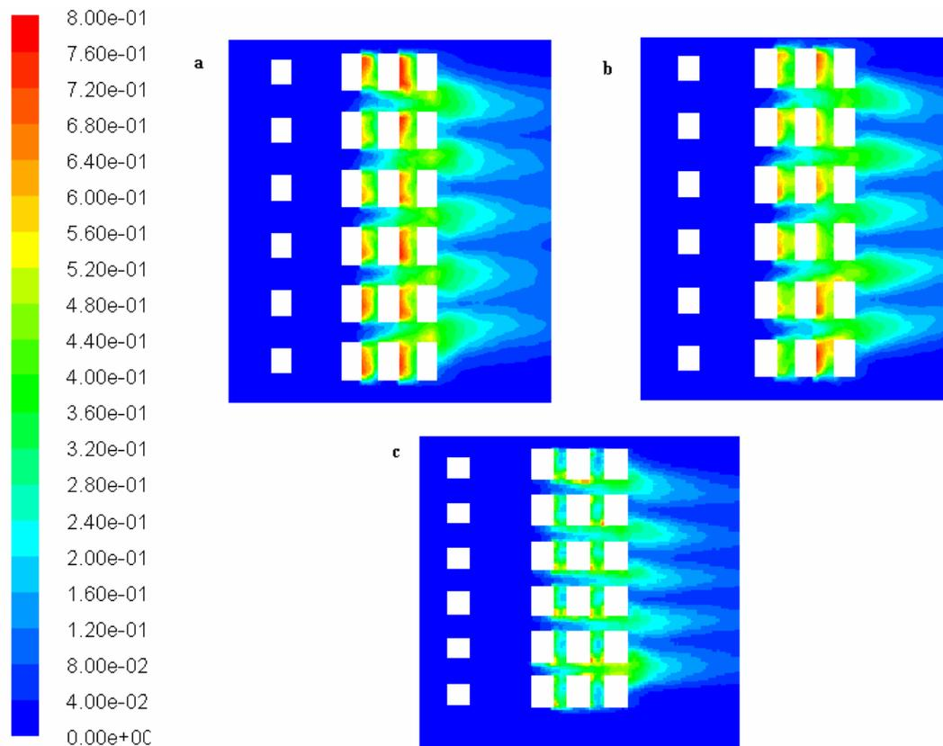
**Figure 10:** NO<sub>2</sub> mol fraction at the pedestrian level (2 m above ground) in case: 26m (a), 32.5(b), 39m(c).
