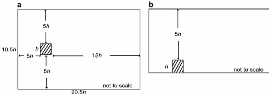
**Figure 2:** Validation case geometry from (a) top view and (b) side view.
