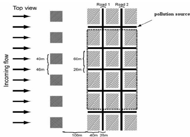
**Figure5:** Top view of building geometry. Black arrows represent wind flow direction.
