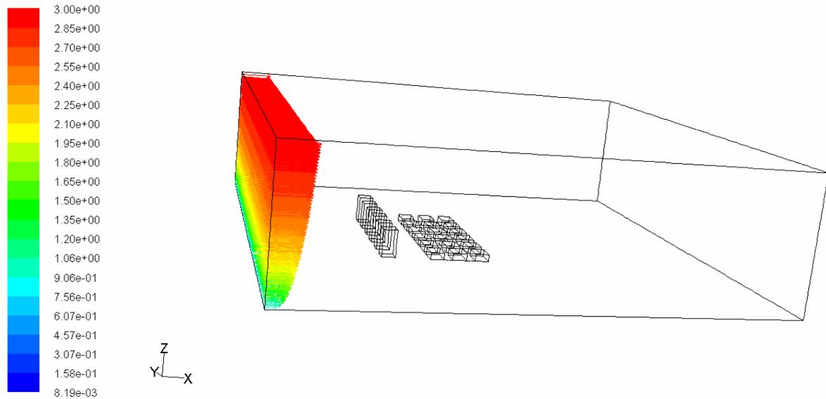
**Figure 6:** wind speed profile for inflow boundary.
