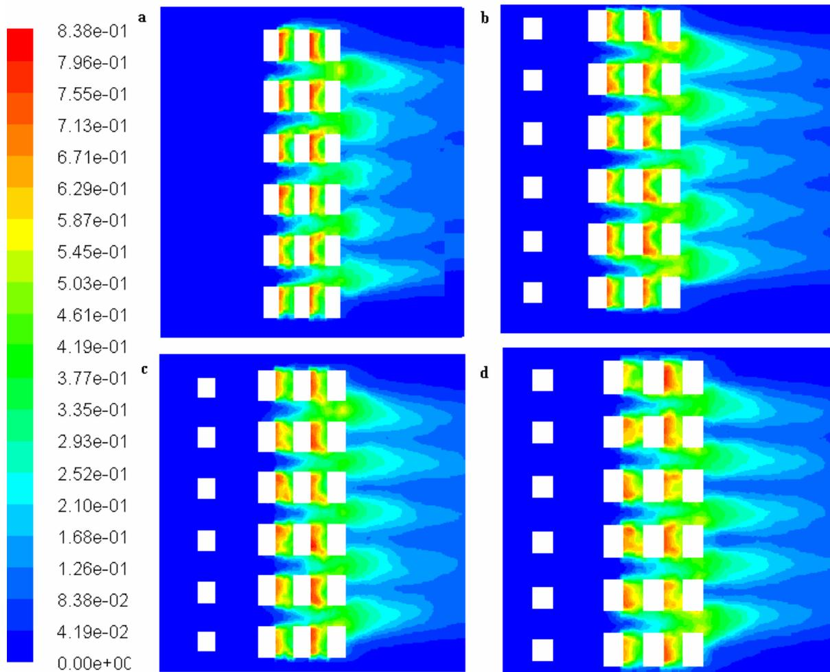
**Figure8:** NO<sub>2</sub> concentration at pedestrian level (2 m above ground) in case: reference (a), H (b), 2H(c), 4H (d).
