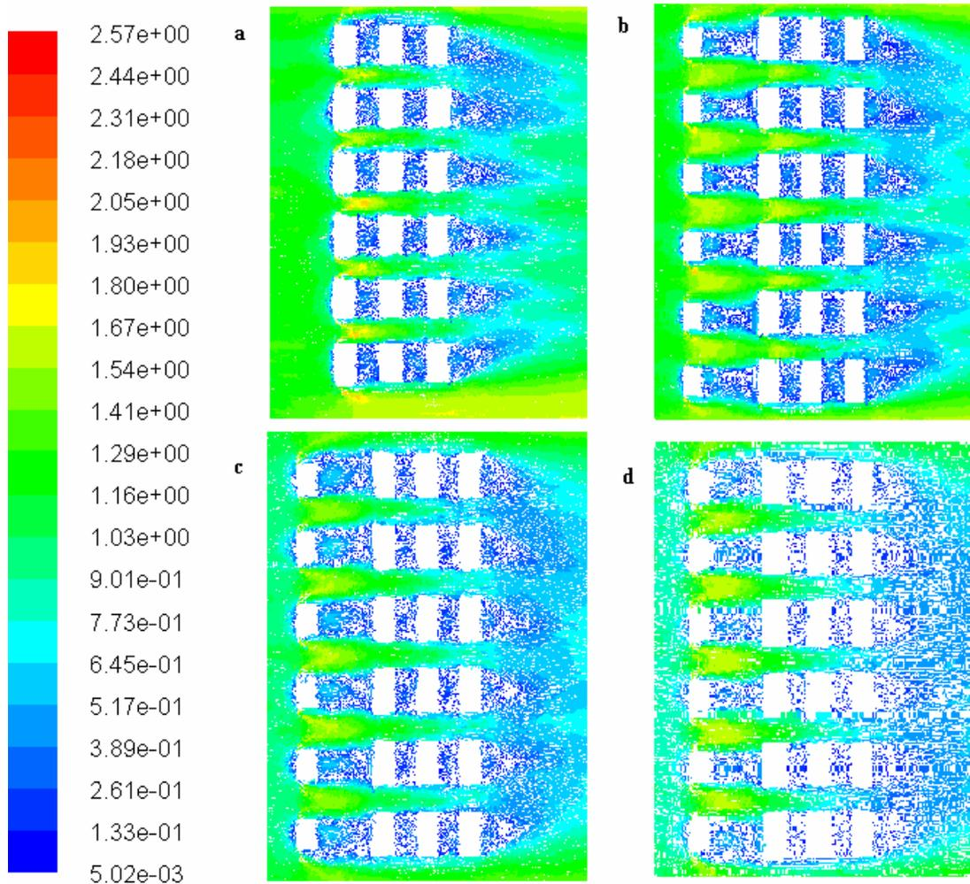
**Figure 9:** velocity vectors at the pedestrian level at pedestrian level (2 m above ground) in case: reference (a), H (b), 2H(c), 4H (d).
