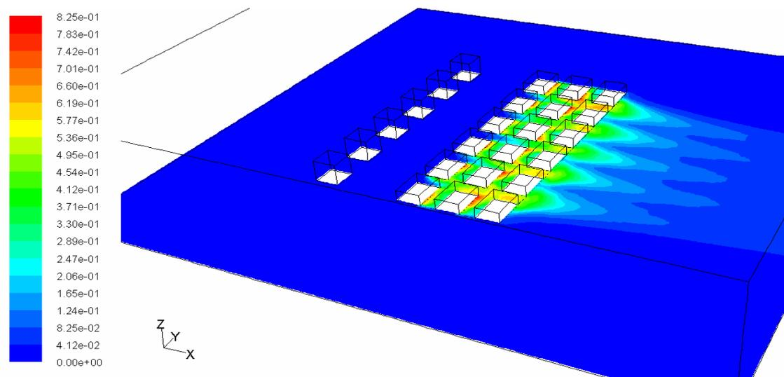
**Figure7:** NO<sub>2</sub> concentration at pedestrian level (2 m above ground)
