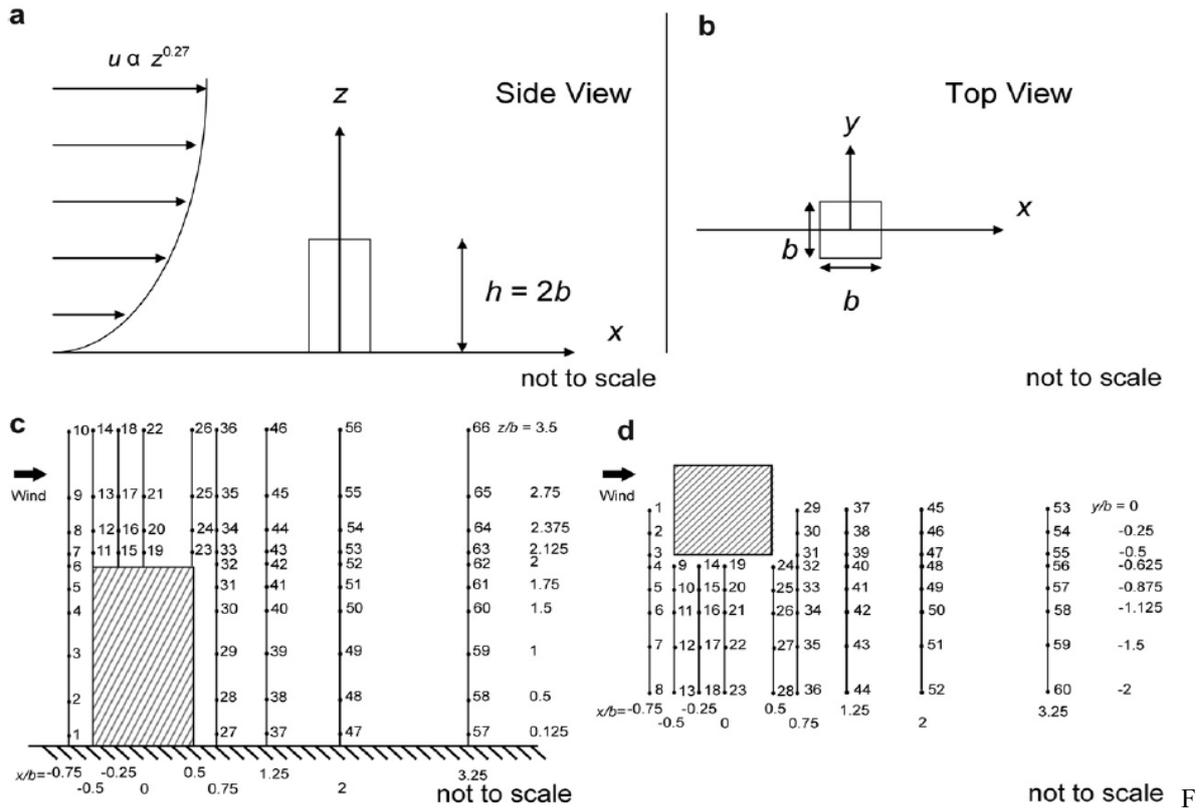
**Figure1:** Configuration of experimental model and approaching wind speed profile from (a) side view and (b) top view. Measurement points in wind tunnel test at (c) centerline on a vertical cross-section and (d) on horizontal planes at  $1/16$  ( $z/b = 0.125$ ) and  $10/16$  ( $z/b = 1.25$ ) of building height.
