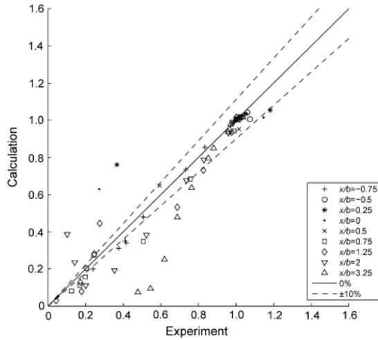
**Figure 3:** Comparison between wind tunnel data and simulation results (Vertical cross section along centerline of building).
