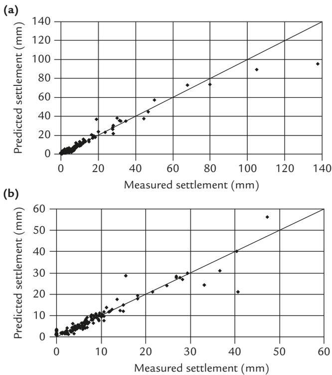
**Figure 1** Measured versus predicted settlements for ANN models with 4 hidden layers with 15-13-5-2 hidden layer nodes: (a) Validation set; and (b) Testing set.
