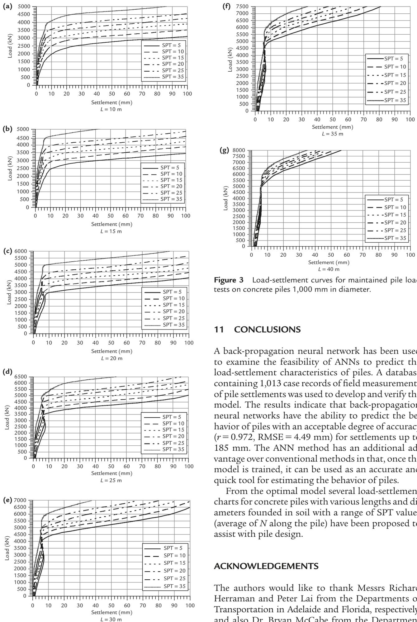
Figure 3 Load-settlement curves for maintained pile load tests on concrete piles 1,000 mm in diameter.
