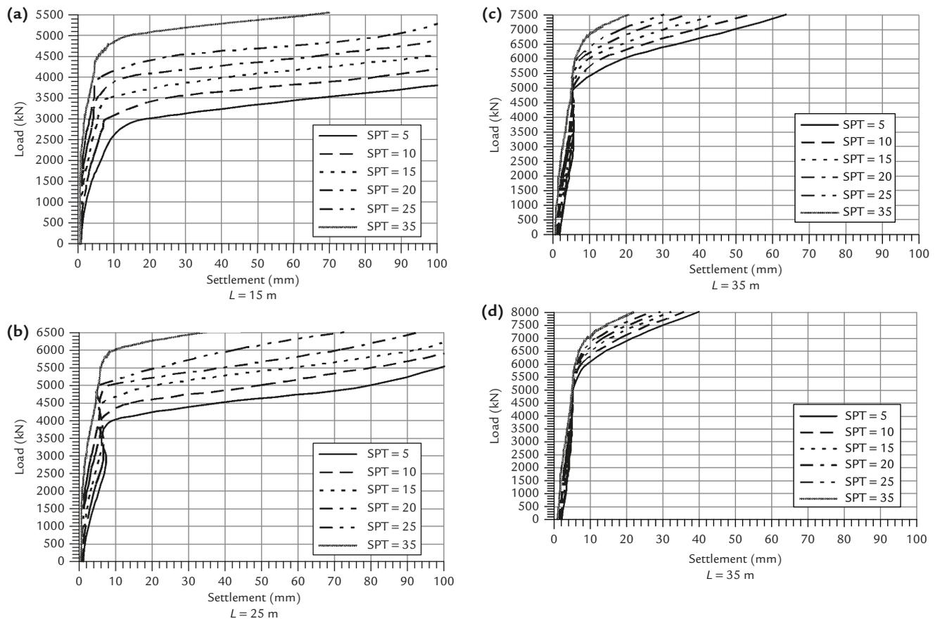
**Figure 4** Load-settlement curves for maintained pile load tests on concrete piles 1,200 mm in diameter.
