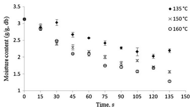
**Fig. 2** Temperature effect on mean moisture change in microwave precooked samples (5.23 W/g)
