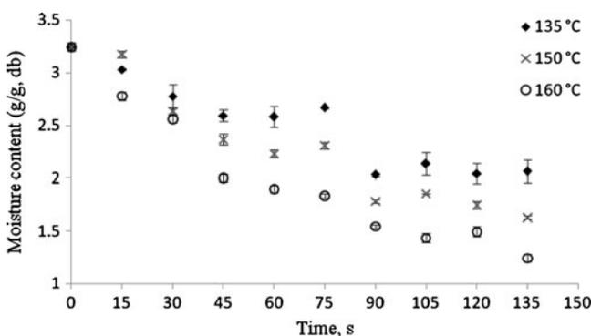
**Fig. 1** Temperature effect on mean moisture change in unprecooked samples
