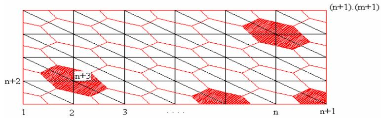
Figure 7. Discretised domain in the FVM
