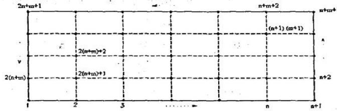
Figure 6. Discretised domain in the BEM
