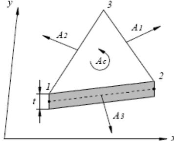
Figure 7. Geometry values of a triangular cell.
