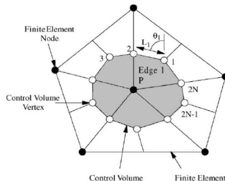
Figure 1. Volume made up of triangular cells
