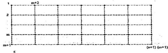
Figure 8. Discretised domain in the EFGM
