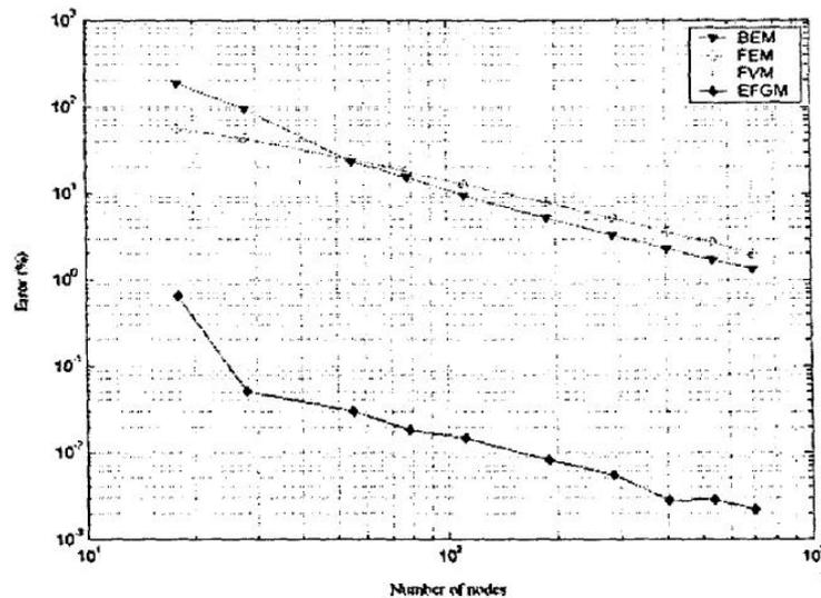
Figure 5. Displacement error for the point A versus the number of nodes
