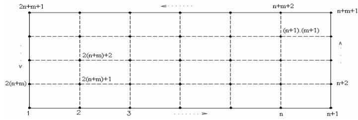
Figure 6. Discretised domain in the BEM
