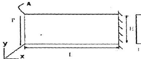
Figure 4. Cantilever beam with the end loading
