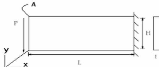
Figure 8. Cantilever beam with the end loading
