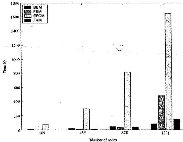
Figure 7. Expended time for the calculation of nodal displacements
