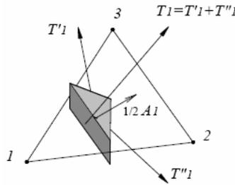
Figure 7. Forces corresponding to the node  $i$  of the cell
