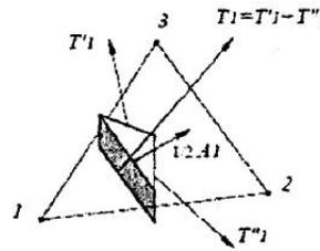
Figure 3. Forces corresponding to the node 1 of the cell
