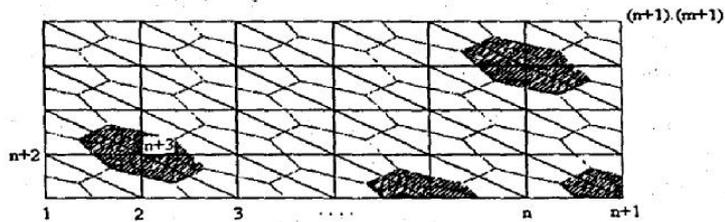
Figure 7. Discretised domain in the FVM
