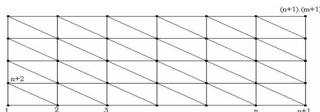
Figure 9. Discretised domain in the FEM
