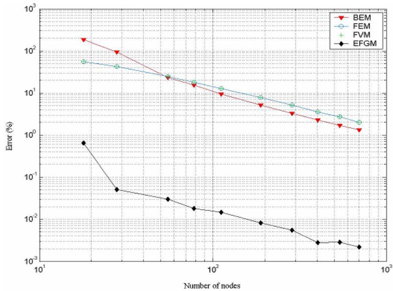
**3-1 Node numbers effect.** A closed form solution to this problem has been given by Timoshenko and Goodier (1951). The percentage of the error in the displacement of point A (see Figure 1) as per different numerical techniques is depicted in Figure 2.
