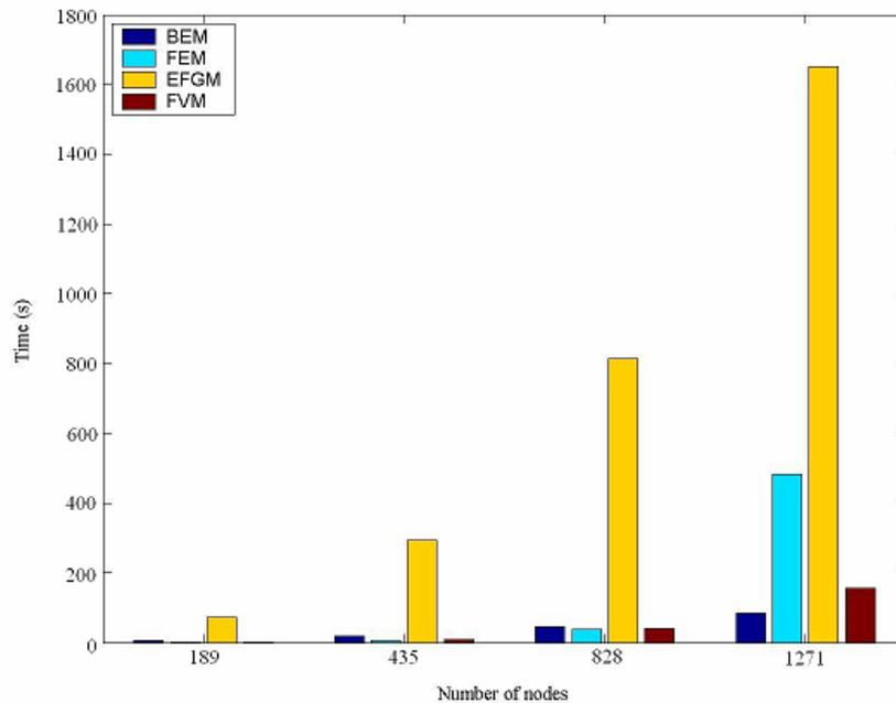
Figure 5. Expended time for the calculation of nodal displacements
