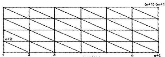
Figure 5. Discretised domain in the FEM
