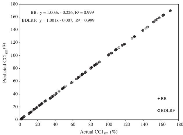
Fig. 9. Predicted values of Artificial Neural Network versus actual values of  $CCI_{rm}$  for BB and BDLRF training algorithms.
