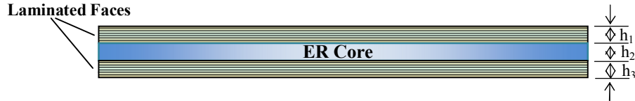
Figure 1: sandwich beam with ER core and laminated faces
