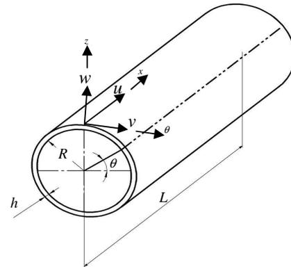
Figure1 : Circular cylindrical shell: coordinate system and dimensions.
