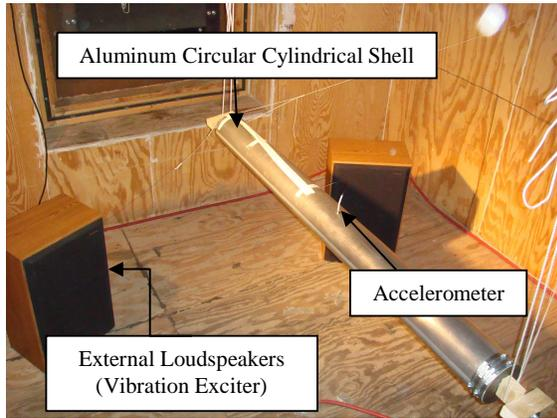
Figure 2: Experimental setup in a reverberant room.
