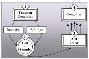
Fig. 1.General synopsis of the experimental apparatus.
