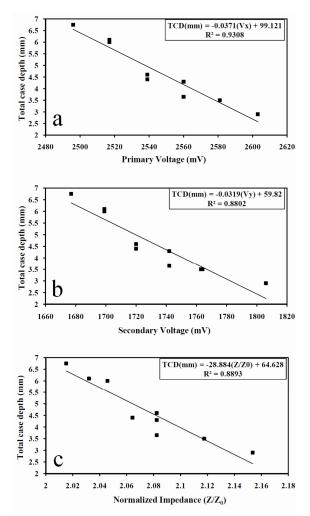
Figure 4: Relations between eddy current outputs and total case depth of the samples.
