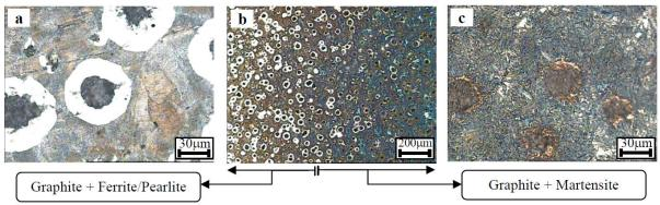
Figure 2: a) Microstructure of the core (ferrite-pearlite and graphite), b) The boundary between the hardened zone near the surface and the core of the material, c) Hardened layer (mirtensite and graphite).
