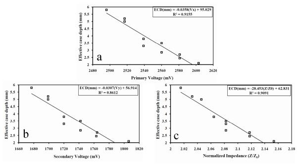
Figure 3: Relations between eddy current outputs and effective case depth of the samples.
