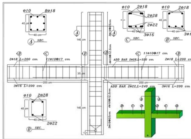
Figure 1. Dimensions and reinforcement details of Monolithic Specimen
