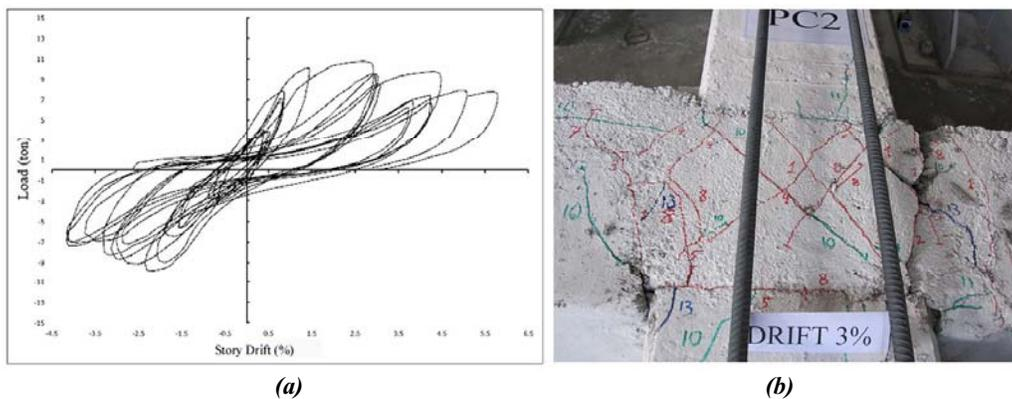
**Figure 8.** (a) Lateral load versus story drift hysteresis response for Specimen PC2
