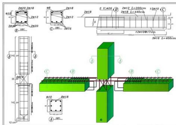
Figure 3. Dimensions and reinforcement details of Specimen PC2
