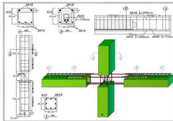
Figure 2. Dimensions and reinforcement details of Specimen PC1
