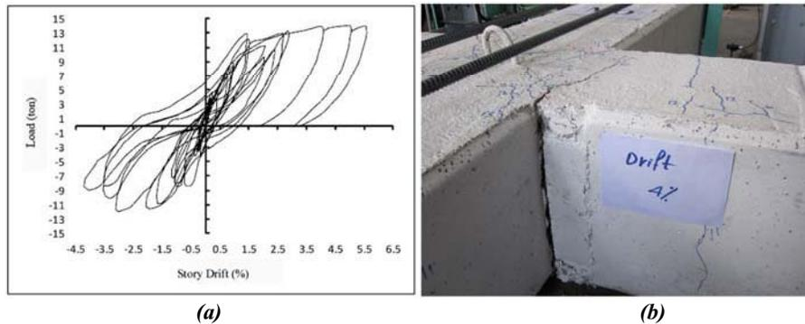
**Figure 6.** (a) Lateral load versus story drift for monolithic specimen
