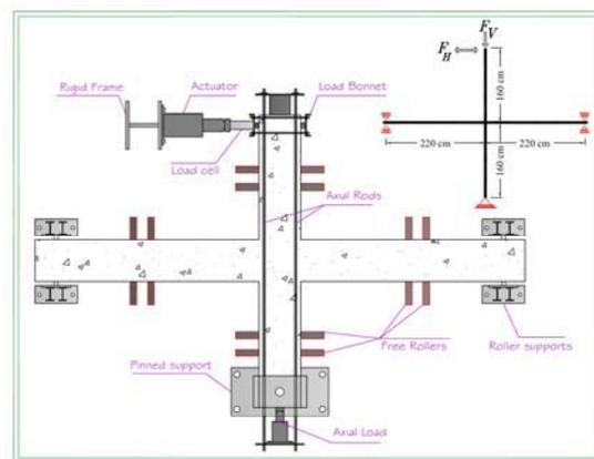
**Figure 4.** Test setup and instrumentations
