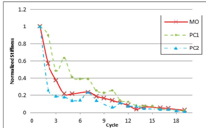
Figure 9. Stiffness degradation of specimens
