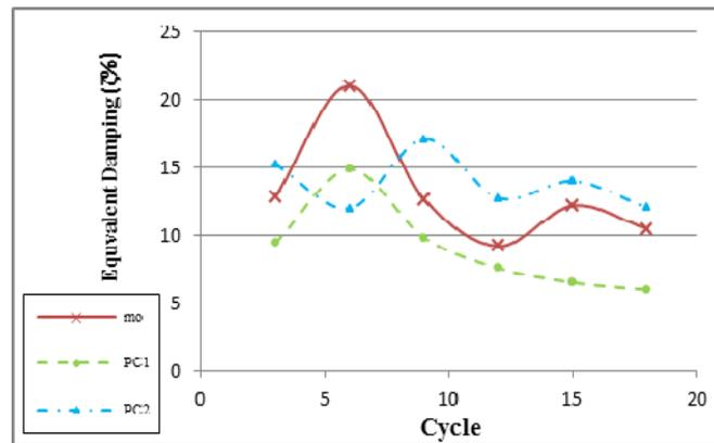
Figure 12. Equivalent damping ratio versus number of cycles for specimens
