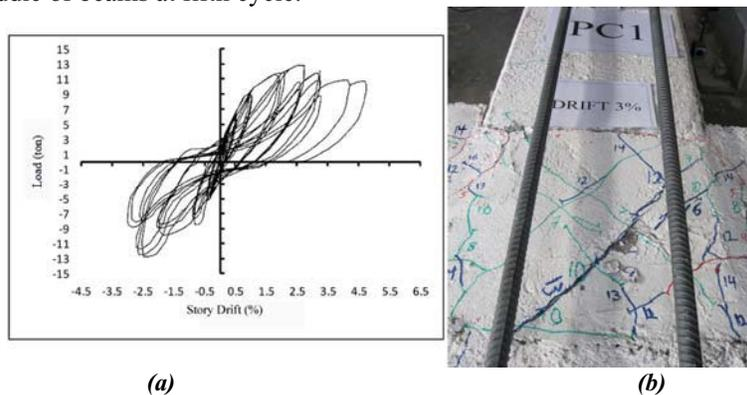
**Figure 7.** (a) Lateral load versus story drift for PC1 specimen
