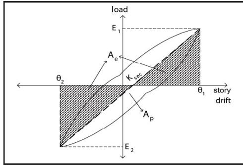
Figure 11. Representation of equivalent damping ratio [2]
