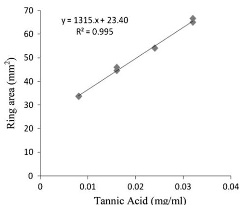
Fig. 1. Calibration curve for tannic acid. Ring areas ( $\text{mm}^2$ ) are regressed against known tannic acid concentrations (mg/ml).
