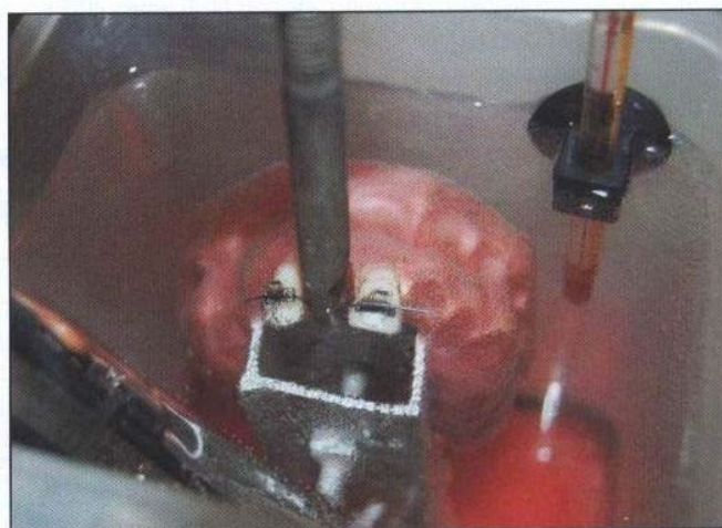
Fig 3. Close up view of the modified three-point bending model on the phantom head jaw with the specimen deflected.
