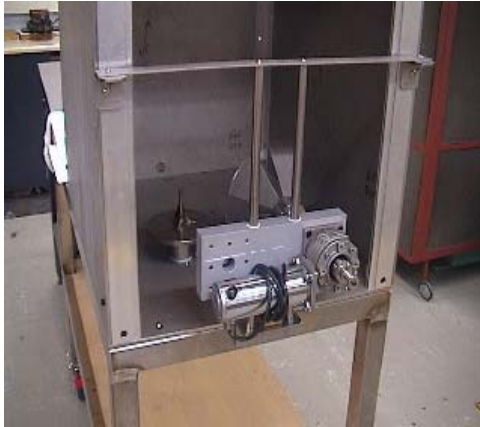
Fig.2a. The chamber of test rig (the drive motor of vegetable holder located at the beneath of chamber)
