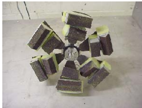
Fig.2d. Assembled peeler head
