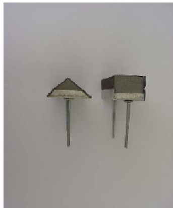
Fig.2c. Abrasive units in different shapes
