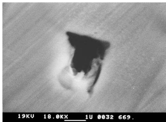
Fig. 9. SEM photomicrograph of a metastable pit in a 904L SS sample after a potentiostatic test at 750 mV (Ag/AgCl) in 1 M NaCl at 49 °C.
