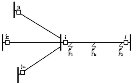
Figure 1 Schematic diagram of Primary and backup relays
